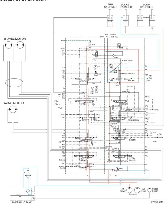
When the right control lever is pulled left, the bucket spool in the main control valve is moved to the roll in position by the pilot oil pressure from the remote control valve.
