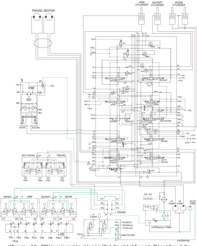
When one of the RCV lever (except travel lever) is tilted, the pilot oil flows into SH port through the main control valve, this pressure move spool so, discharged oil from pilot valve flow into PG port. This pressure is applied to swing motor disc, thus the brake is released.
