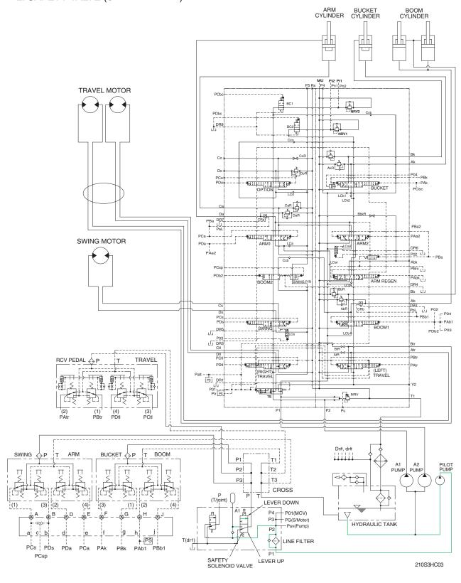
When the lever of the safety solenoid valve is moved downward, oil flows into the remote control valve through solenoid valve and line filter.
