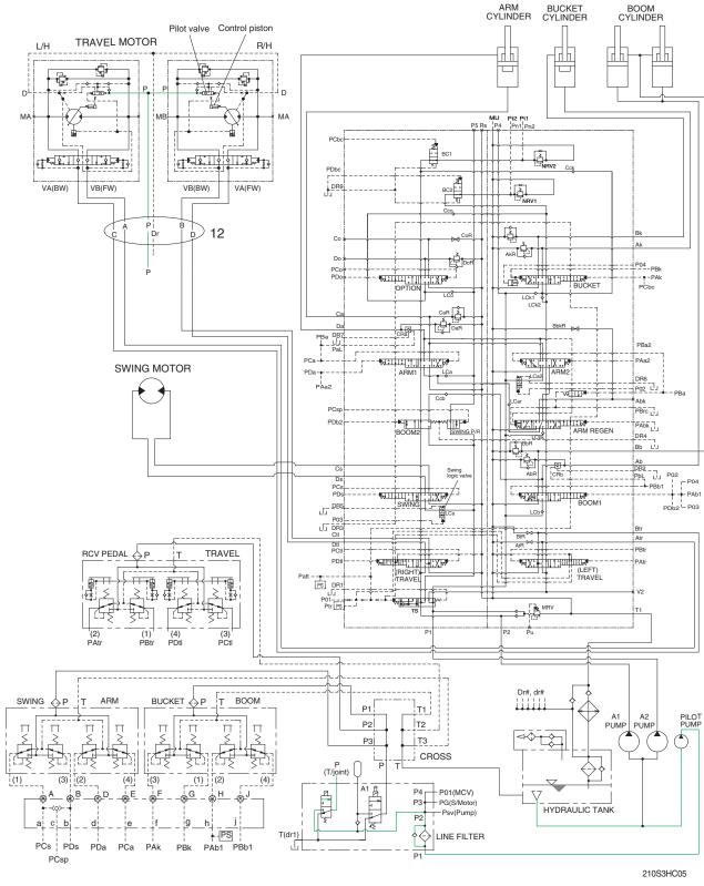
When the travel speed switch is pushed, the travel speed solenoid valve is actuated and the discharged oil from the pilot pump flows to the P port of pilot valve in the travel motors.
