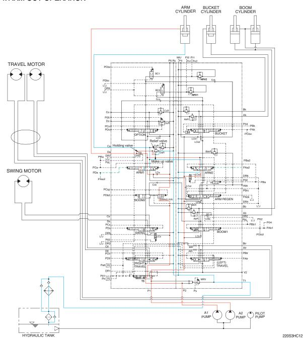
When the left control lever is pushed forward, the arm spools in the main control valve are moved to the roll out position by the pilot oil pressure from the remote control valve.
