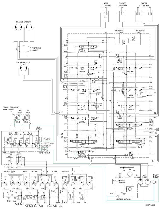
When the travel and other function (boom, arm, bucket, swing, option B or option C) are operated, the travel straight EPPR value is energized by the MCU that senses the pilot pressure of the travel and other functions and Pd0 pressure from the travel straight EPPR value changes the travel straight spool.
