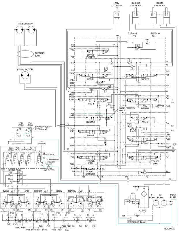
When carrying out the combined operation of swing and arm in of the left control valve, the swing speed can be lowered than operating speed of arm.
