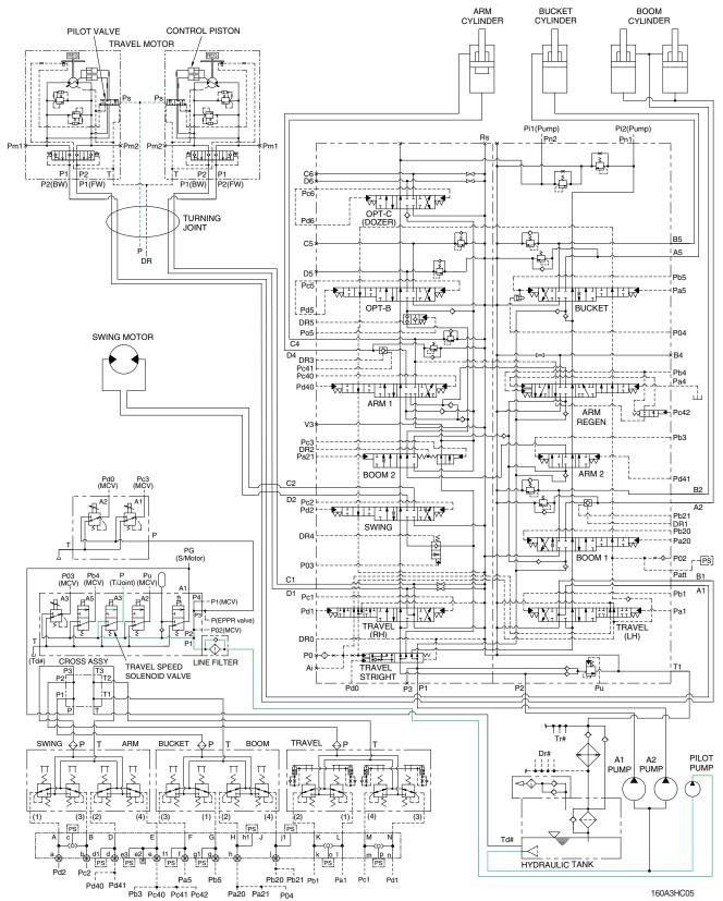
When the travel speed solenoid valve was placed in the Hi position, the pressure oil from pilot pump through line filter flows to port **Ps** of travel speed change over valve, and the control piston is pushed left (LH) and right (RH), thus minimizing the displacement.
