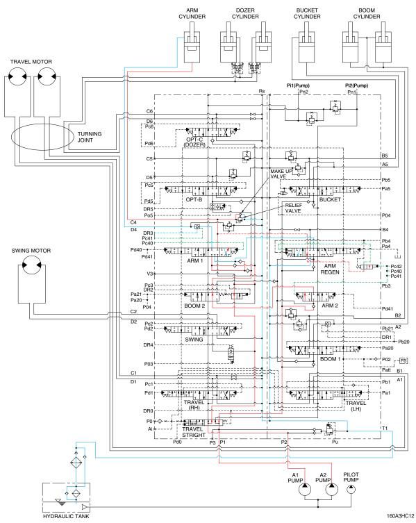
When the left control lever is pulled back, the arm spools in the main control valve are moved to the roll in position by the pilot oil pressure (Pc40, Pb3) from the remote control valve.
