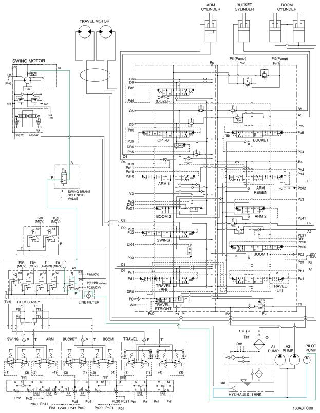
When any of the swing, arm in, boom up or travel is tilted, the swing brake solenoid valve is shifted to the downward by the MCU that senses the pilot pressure of the swing control lever.
