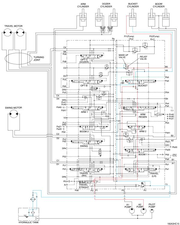
When the right control lever is pushed right, the bucket spool in the main control valve is moved to the roll out position by the pilot oil pressure (Pb5) from the remote control valve.
