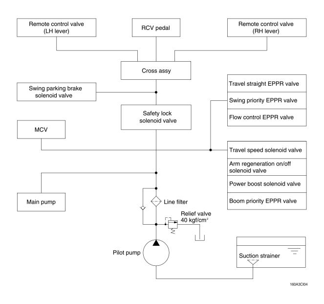
The pilot circuit consists of suction circuit, delivery circuit and return circuit.
