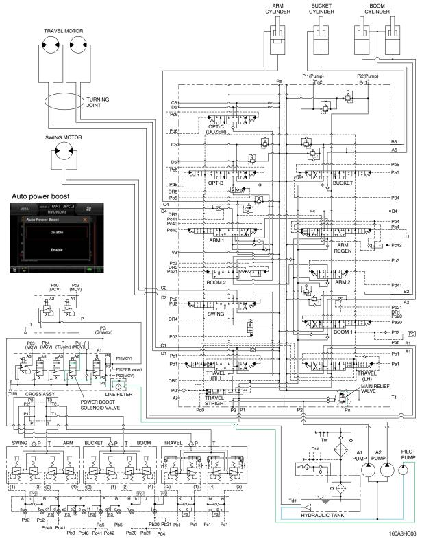
When the power boost switch on the left control lever is pushed ON, the power boost solenoid valve is actuated, the discharged oil from the pilot pump flows into **Pu** port of the main relief valve of main control valve; then the setting pressure of the main relief valve is raised from 350 kgf/cm<sup>2</sup> (4980 psi) to 380 kgf/cm<sup>2</sup> (5400 psi) for increasing the digging power.
