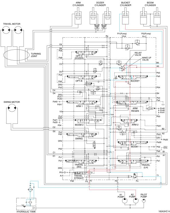
When the right control lever is pulled left, the bucket spool in the main control valve is moved to the roll in position by the pilot oil pressure (Pa5) from the remote control valve.
