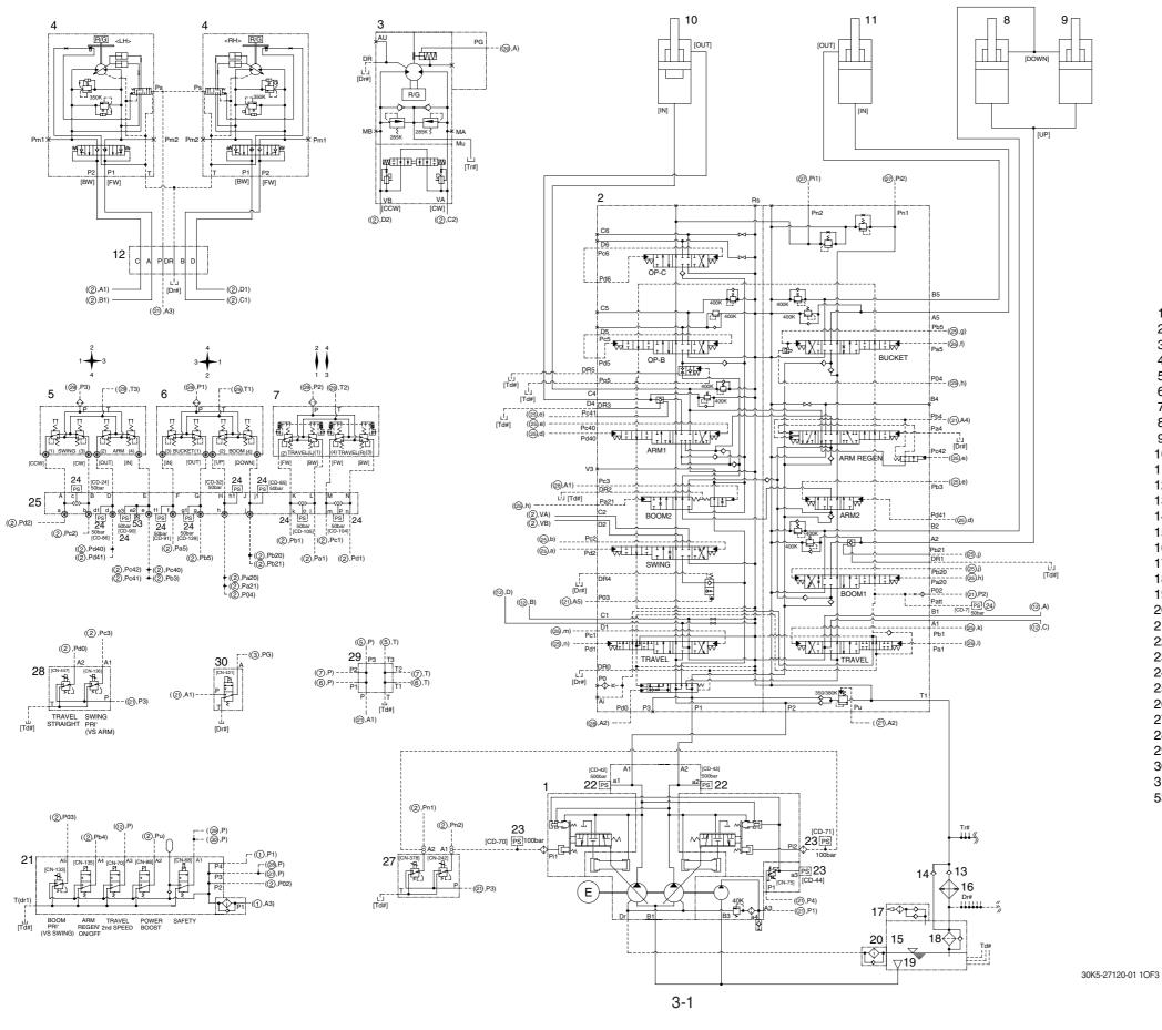
3 Swing motor 4 Travel motor RCV lever (LH) 5 RCV lever (RH) 6 RCV pedal 7 Boom cylinder (LH) 8 Boom cylinder (RH) 9
