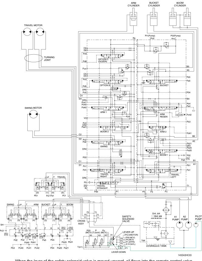
When the lever of the safety solenoid valve is moved upward, oil flows into the remote control valve through line filter solenoid valve and cross assy.
