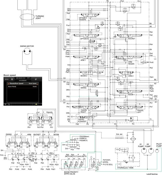
When carrying out the combined operation of swing and boom up, the boom up operating speed is lowered then normal operation.
