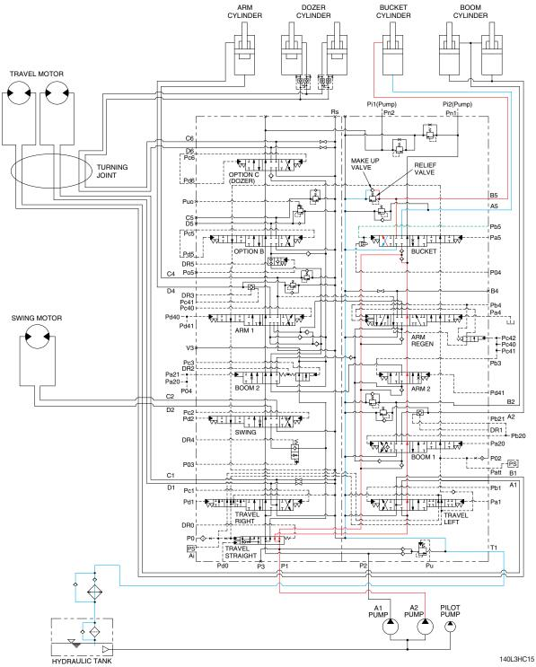
When the right control lever is pushed right, the bucket spool in the main control valve is moved to the bucket out position by the pilot oil pressure (Pb5) from the remote control valve.
