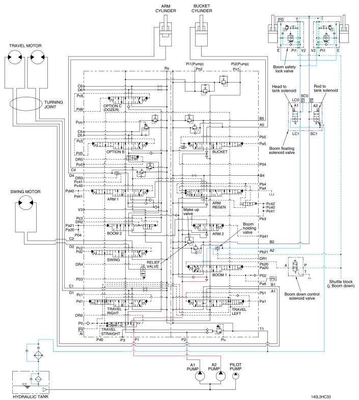
When the travel and other functions (boom, arm, bucket, swing, option) are tilted, the travel straight EPPR valve is energized by the MCU that senses the pilot pressure of the travel and other functions and Pd0 pressure from the travel straight EPPR valve changes the travel straight spool.
