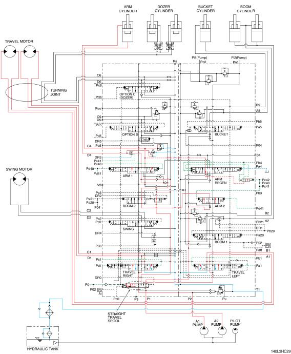
When the arm and travel functions are operated simultaneously, the arm spools and travel spools in the main control valve are moved to the functional position by the pilot oil pressure (Pc40, Pb3, Pd40, Pd41, Pa1, Pb1, Pc1, Pd1) from the remote control valve and the straight travel spool is pushed to the right by the oil pressure of the travel straight EPPR valve.
