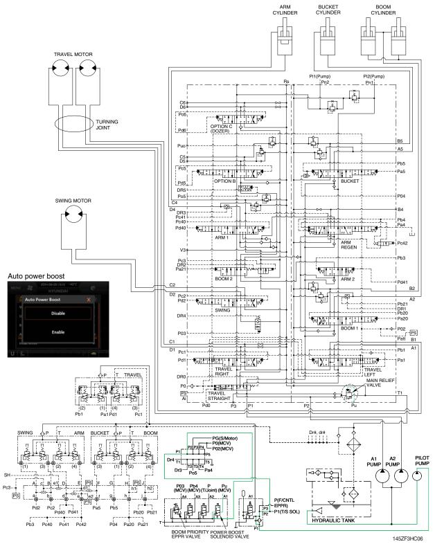
When the power boost switch on the left control lever is pushed ON, the power boost solenoid valve is actuated, the discharged oil from the pilot pump flows into **Pu** port of the main relief valve of main control valve; then the setting pressure of the main relief valve is raised from 350 kgf/cm<sup>2</sup> (4980 psi) to 380 kgf/cm<sup>2</sup> (5400 psi) for increasing the digging power.
