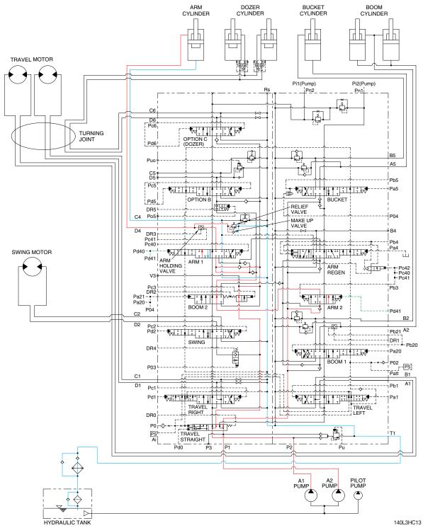
When the left control lever is pushed forward, the arm spools in the main control valve are moved to the arm out position by the pilot oil pressure (Pd40, Pd41) from the remote control valve.
