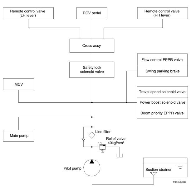
The pilot circuit consists of suction circuit, delivery circuit and return circuit.
