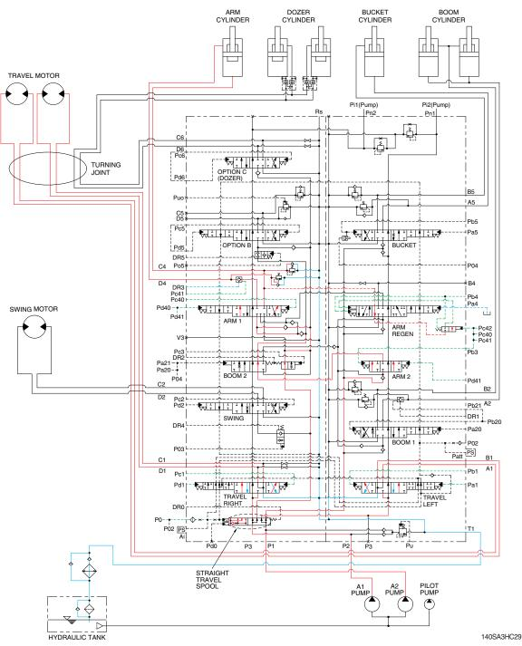
When the arm and travel functions are operated simultaneously, the arm spools and travel spools in the main control valve are moved to the functional position by the pilot oil pressure (Pc40, Pd40, Pd41, Pb3, Pc2, Pd2, Pa1, Pb1, Pc1, Pd1) from the remote control valve and the straight travel spool is pushed to the right by the oil pressure (P0, P01) from pilot pump.
