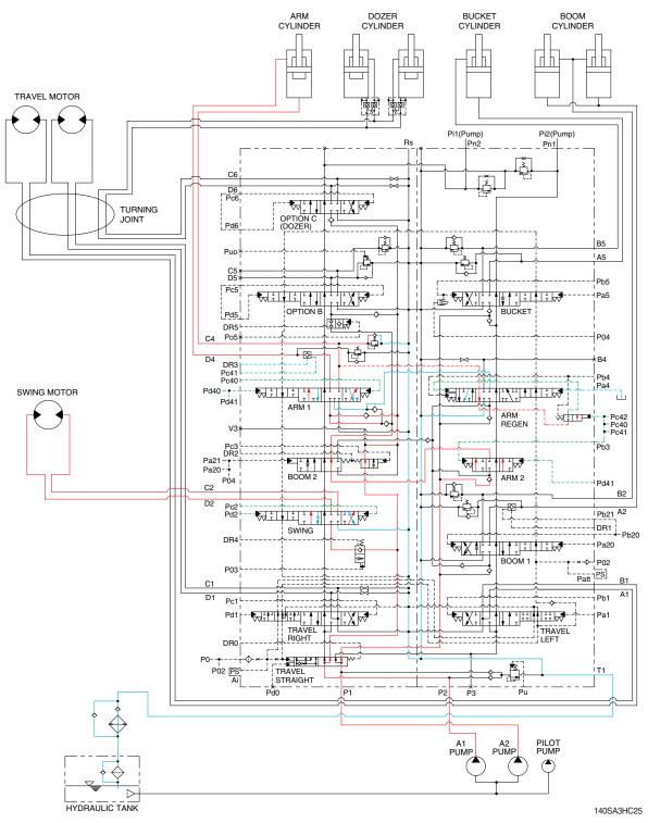
When the swing and arm functions are operated simultaneously, the swing spool and arm spools in the main control valve are moved to the functional position by the pilot oil pressure (Pc2, Pd2, Pc40, Pd40, Pd41, Pb3) from the remote control valve.
