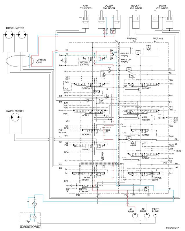
When the dozer control lever is pushed forward, the dozer spool in the main control valve is moved to the dozer down position by the pilot oil pressure (Pc6) from the remote control valve.
