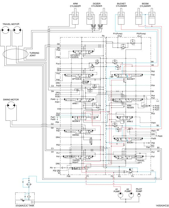
When the boom up and bucket in functions are operated simultaneously, each spool in the main control valve is moved to the functional position by the pilot oil pressure (Pa20, Pa21, Pa5) from the remote control valve.
