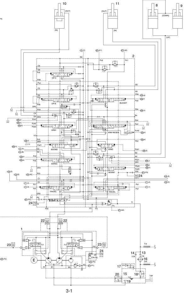
Main pump Main control valve Swing motor Travel motor RCV lever (LH) RCV lever (RH) RCV pedal Boom cylinder (LH) Boom cylinder (RH) 10 Arm cylinder Bucket cylinder Turning joint Return check valve Return check valve Hydraulic tank 16 Oil cooler 17 Air breather 18 Return filter w/bypass valve Strainer Drain filter 4-cartridge valve Pressure sensor Pressure sensor Pressure sensor Terminal block Last guard filter 2-EPPR valve 29 Cross assy
