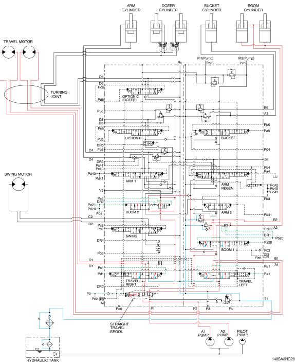
When the boom and travel functions are operated simultaneously, the boom spools and travel spools in the main control valve are moved to the functional position by the pilot oil pressure (Pa20, Pa21, Pc2, Pd2, Pa1, Pb1, Pc1, Pd1) from the remote control valve and the straight travel spool is pushed to the right by the oil pressure (P0, P01) from pilot pump.
