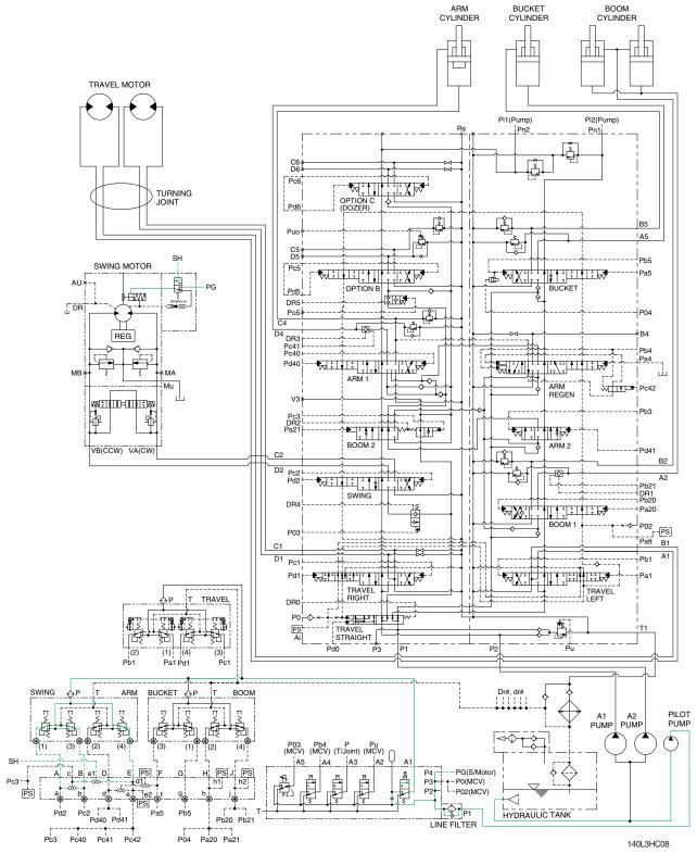
When any lever of the swing, arm in, boom up or travel is tilted, the swing brake solenoid valve is shifted to the downward by the MCU that senses the pilot pressure of the RCV control lever.
