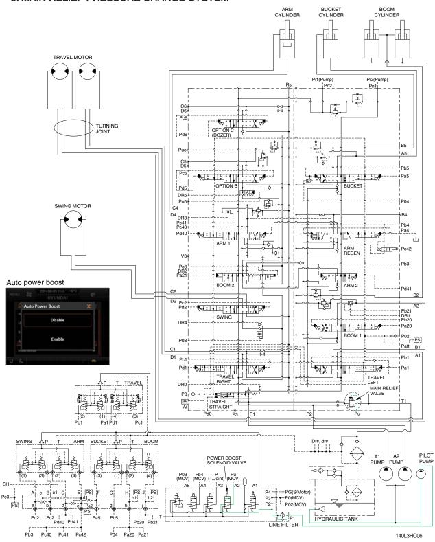
When the power boost switch on the left control lever is pushed ON, the power boost solenoid valve is actuated, the discharged oil from the pilot pump flows into **Pu** port of the main relief valve of main control valve; then the setting pressure of the main relief valve is raised from 350 kgf/cm² to 380 kgf/cm² for increasing the digging power.
