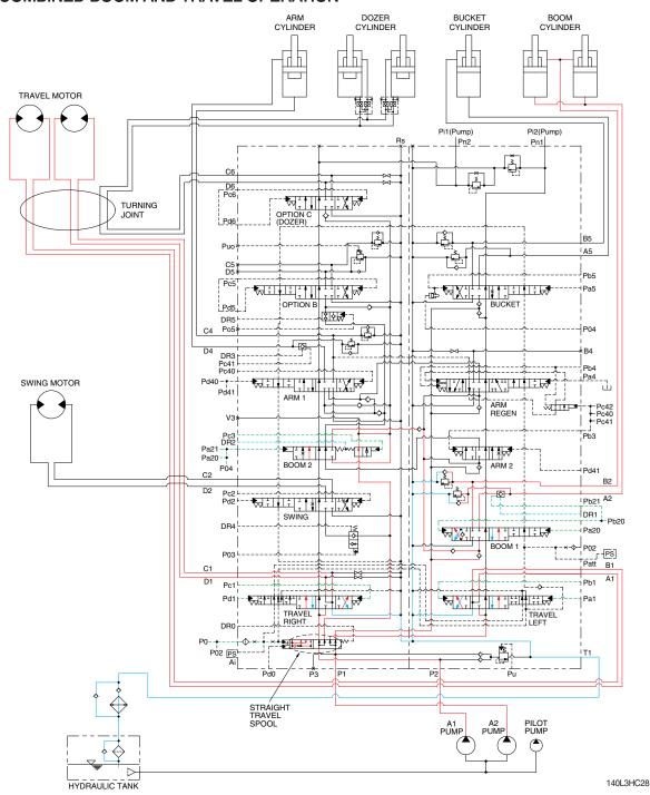
When the boom and travel functions are operated simultaneously, the boom spools and travel spools in the main control valve are moved to the functional position by the pilot oil pressure (Pa20, Pa21, Pb20, Pc2, Pd2, Pa1, Pb1, Pc1, Pd1) from the remote control valve and the straight travel spool is pushed to the right by the oil pressure of the travel straight EPPR valve.
