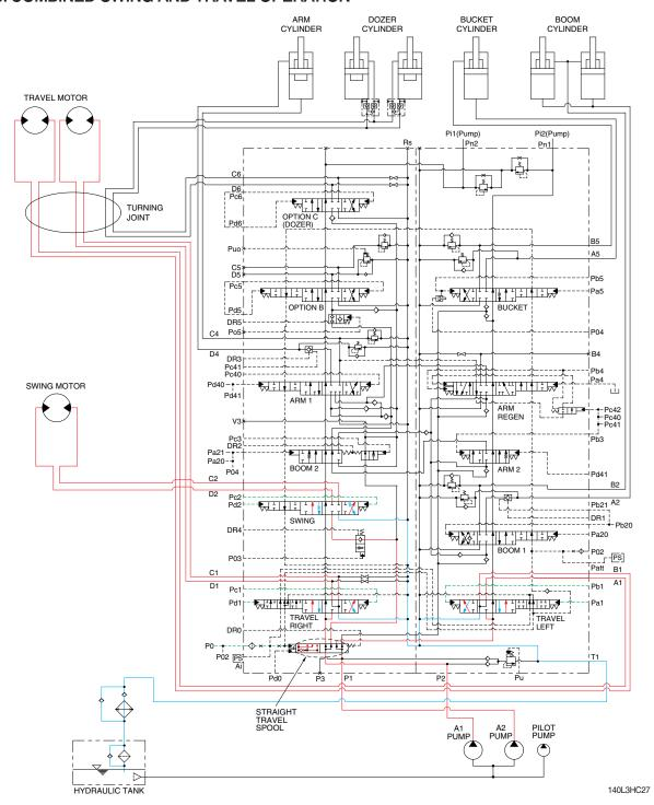
When the swing and travel functions are operated simultaneously, the swing spool and travel spools in the main control valve are moved to the functional position by the pilot oil pressure (Pc2, Pd2, Pa1, Pb1, Pc1, Pd1) from the remote control valve and straight travel spool is pushed to the right by the pilot oil pressure of the travel straight EPPR valve.
