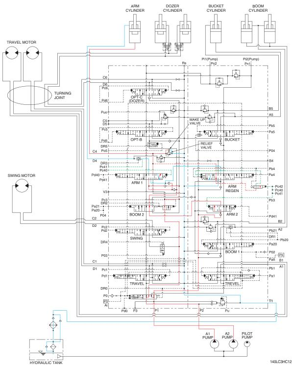
When the left control lever is pulled back, the arm spools in the main control valve are moved to the arm in position by the pilot oil pressure from the remote control valve.
