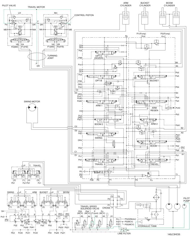
When the travel speed solenoid valve was placed in the Hi position, the pressure oil from pilot pump through line filter flows to port **Ps** of travel speed change over valve, and the control piston is pushed left and right, thus minimizing the displacement.
