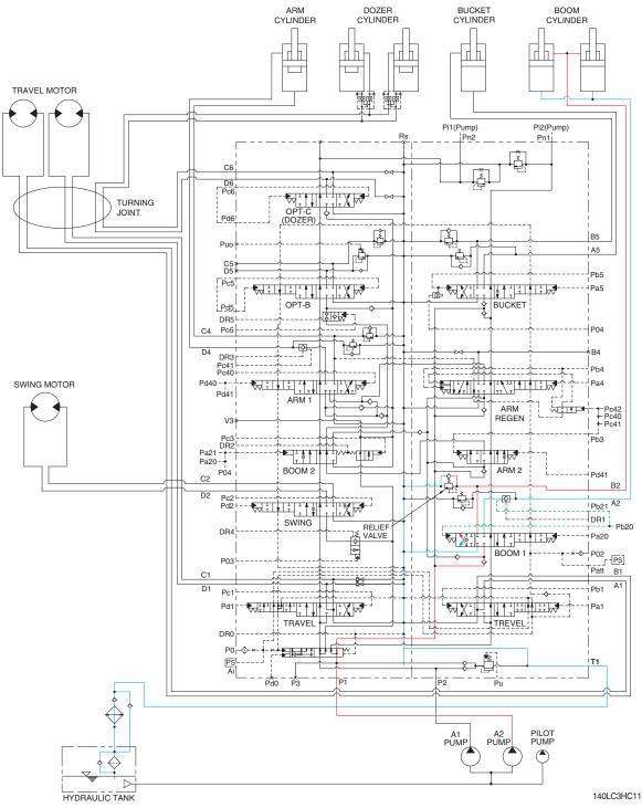
When the right control lever is pushed forward, the boom 1 spool in the main control valve is moved to the down position by the pilot oil pressure from the remote control valve.
