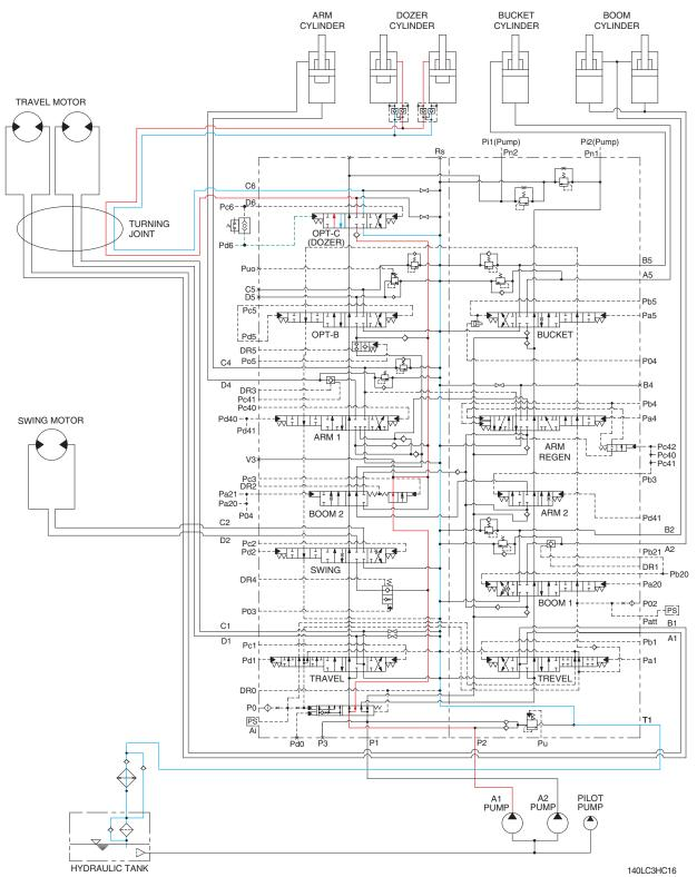
When the dozer control lever is pulled back, the dozer spool in the main control valve is moved to the dozer up position by the pilot oil pressure from the remote control valve.
