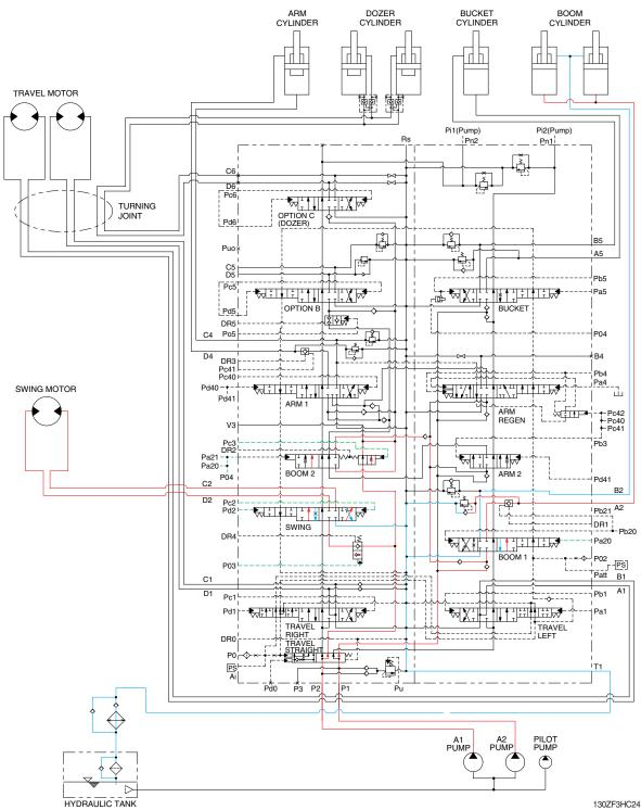
When the swing and boom up functions are operated simultaneously, the swing spool and boom spools in the main control valve are moved to the functional position by the pilot oil pressure (Pc2, Pd2, Pa20, Pa21) from the remote control valve.
