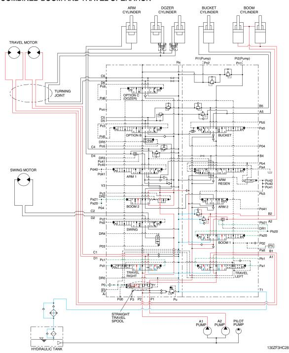
When the boom and travel functions are operated simultaneously, the boom spools and travel spools in the main control valve are moved to the functional position by the pilot oil pressure (Pa20, Pa21, Pb20, Pc2, Pd2, Pa1, Pb1, Pc1, Pd1) from the remote control valve and the straight travel spool is pushed to the right by the oil pressure from pilot pump.
