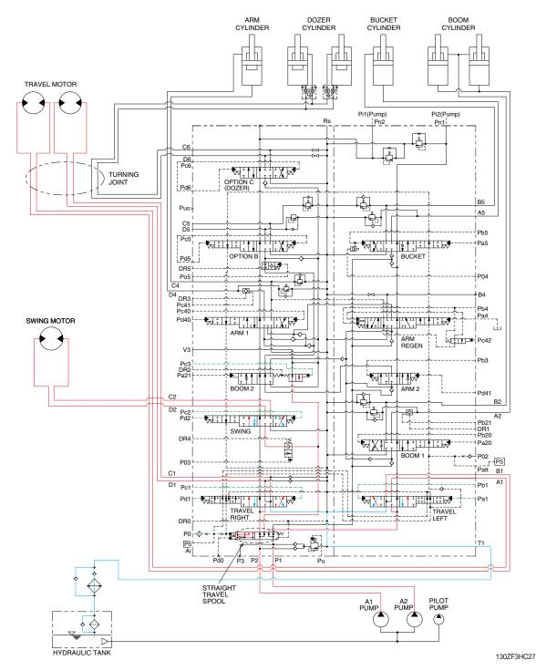
When the swing and travel functions are operated simultaneously, the swing spool and travel spools in the main control valve are moved to the functional position by the pilot oil pressure (Pc2, Pd2, Pa1, Pb1, Pc1, Pd1) from the remote control valve and straight travel spool is pushed to the right by the pilot oil pressure from the pilot pump.
