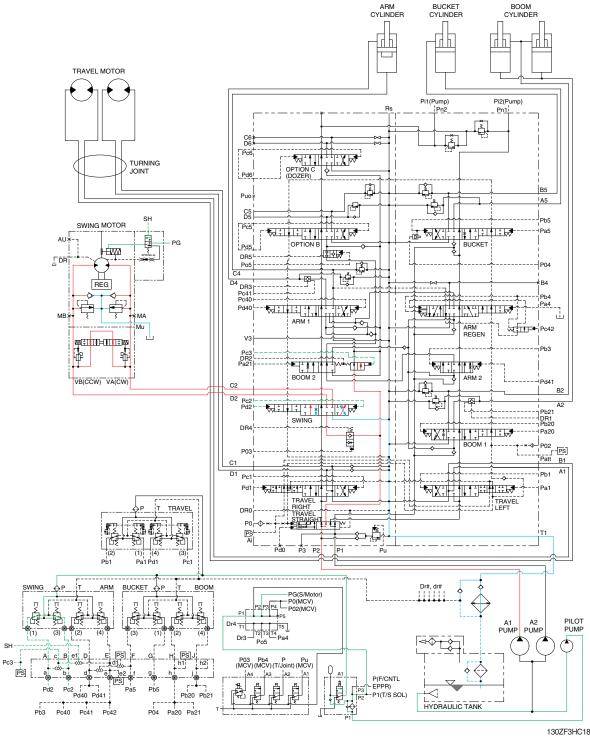
When the left control lever is pushed left or right, the swing spool in the main control valve is moved to the left or right swing position by the pilot oil pressure (Pc2, Pd2) from the remote control valve. Also the swing operation preference function is operated by the pilot pressure **Pc3** (refer to page 3-15).
