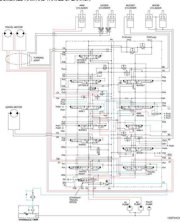
When the arm and travel functions are operated simultaneously, the arm spools and travel spools in the main control valve are moved to the functional position by the pilot oil pressure (Pc40, Pb3, Pd40, Pd41, Pa1, Pb1, Pc1, Pd1) from the remote control valve and the straight travel spool is pushed to the right by the oil pressure from pilot pump.
