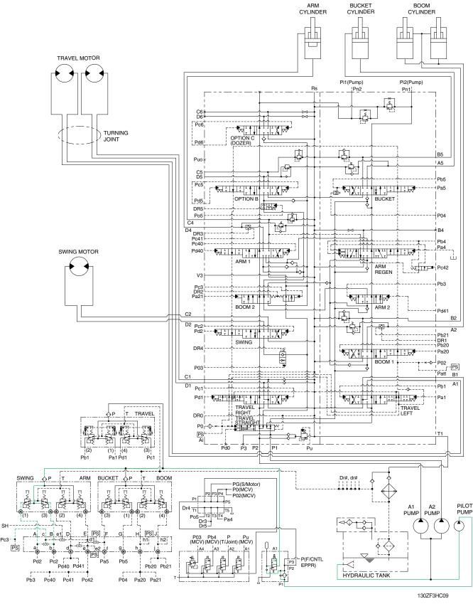
When the swing and arm in control levers are tilted simultaneously, the swing priority EPPR valve is energized by the MCU that senses the swing pilot pressure and Pc3 pressure from the swing priority EPPR valve change the swing priority spool and decreases the oil flow rate to the next section to make the swing operation most preferential.
