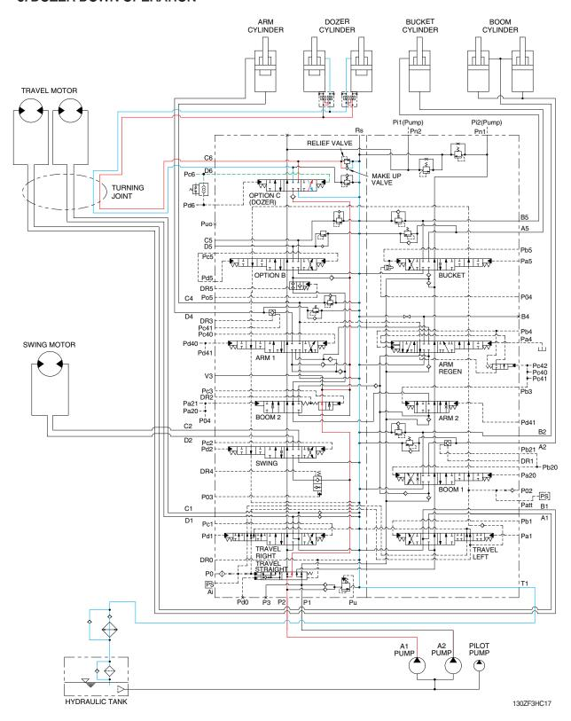
When the dozer control lever is pushed forward, the dozer spool in the main control valve is moved to the dozer down position by the pilot oil pressure (Pc6) from the remote control valve.
