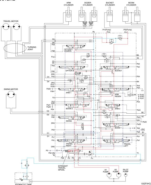
The oil from the A1 and A2 pump flows through the neutral oil passage, bypass oil passage and confluence oil passage in the main control valve. Then the oil goes to each actuator and operates them. Check valves and orifices are located on these oil passage in the main control valve. These control the oil from the main pumps so as to correspond to the operation of each actuator and smooth the combined operation.
