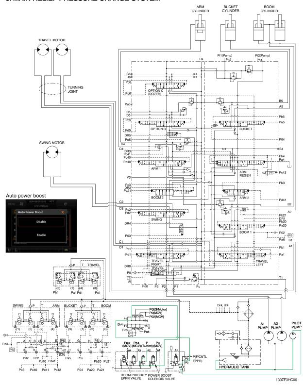
When the power boost switch on the left control lever is pushed ON, the power boost solenoid valve is actuated, the discharged oil from the pilot pump flows into **Pu** port of the main relief valve of main control valve; then the setting pressure of the main relief valve is raised from 330 kgf/cm² (4690 psi) to 360 kgf/cm² (5120 psi) for increasing the digging power.
