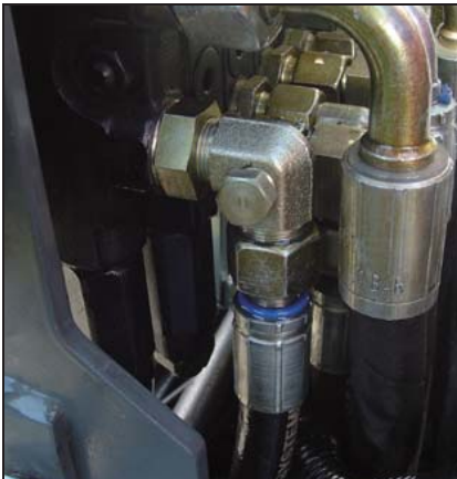
Fig. 28: Plug instead of measurement connection
