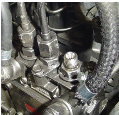
Fig. 8: Opening on fuel pump
