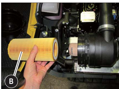
Fig. 22: Removing the outside air filter
