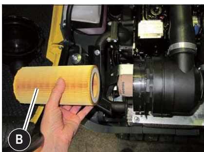
Fig. 24: Removing the outside air filter
