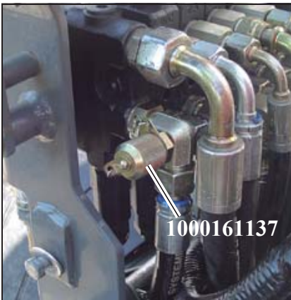
Fig. 29: Secondary pressure limiting valve measurement connection
