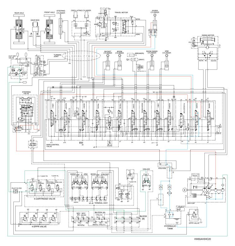
When the dozer control lever is pulled back, the dozer spool in the main control valve is moved to the dozer up position by the pilot oil pressure (b2) from the remote control valve.
