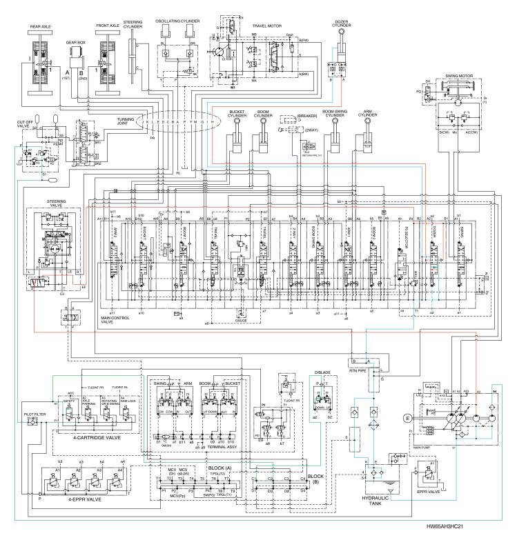
When the dozer control lever is pushed forward, the dozer spool in the main control valve is moved to the dozer down position by the pilot oil pressure (a2) from the remote control valve.
