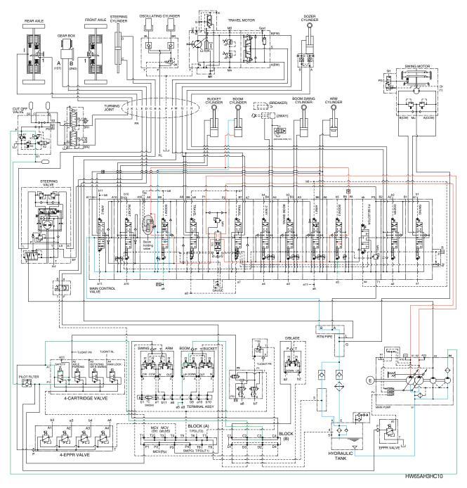
When the right control lever is pulled back, the boom spools in the main control valve are moved to the up position by the pilot oil pressure (a5, a9) from the remote control valve.
