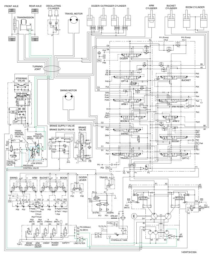
When RH multifunction switch was placed in high or low speed position, the pressure oil from pilot pump flows to travel speed solenoid valve through pressure control valve, thus the transmission is changed into high (P1) or low (P2) speed condition.
