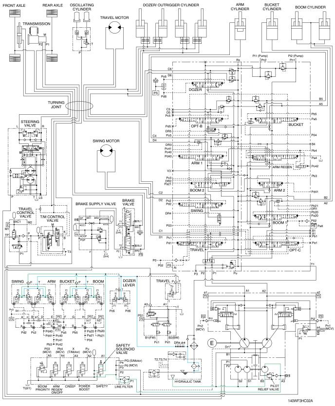
The pilot pump receives oil from the hydraulic tank. The discharged oil from the pilot pump flows to the safety solenoid valve through the line filter. The oil is filtered by the line filter. The pilot relief valve is provided in the pilot pump for limiting the pilot circuit pressure.
