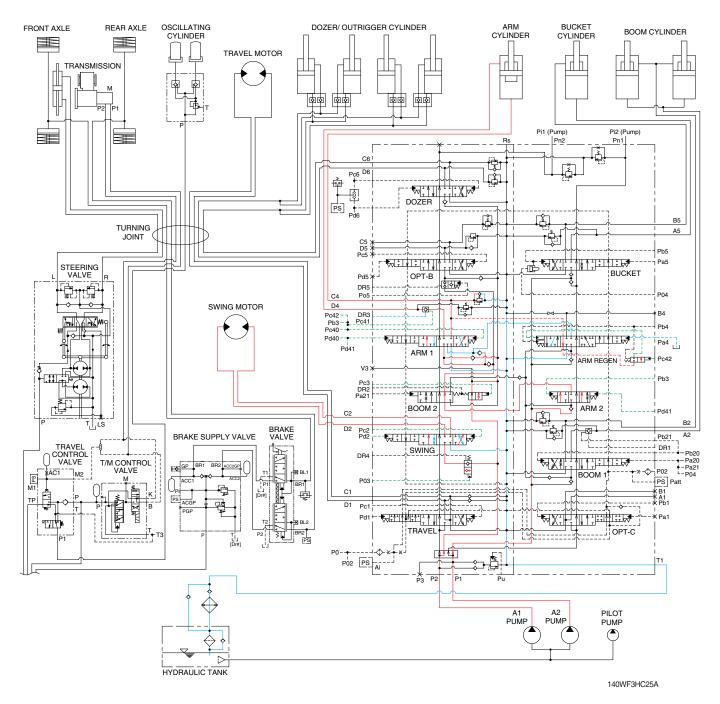
When the swing and arm functions are operated, simultaneously the swing spool and arm spools in the main control valve are moved to the functional position by the pilot oil pressure from the remote control valve.
