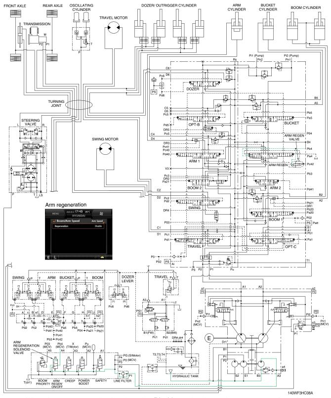
When the arm regeneration is selected to **Disable** on the cluster, the arm regeneration solenoid valve is activated. The pilot oil from pilot pump flows into **Pb4** port in main control valve through solenoid valve and the arm regeneration spool is shifted to right.
