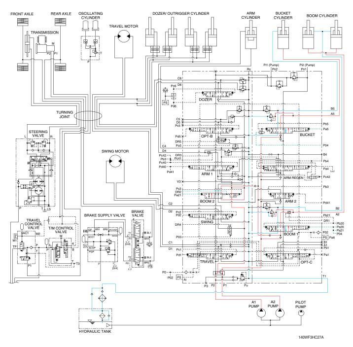
When the boom up and bucket functions are operated simultaneously, each spool in the main control valve is moved to the functional position by the pilot oil pressure from the remote control valve.
