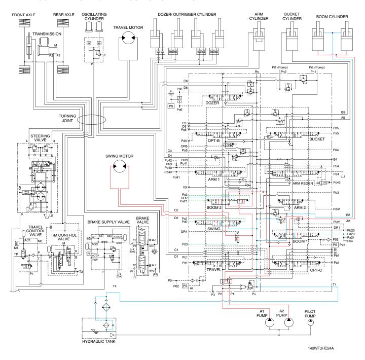
When the swing and boom up functions are operated, simultaneously the swing spool and boom spools in the main control valve are moved to the functional position by the pilot oil pressure from the remote control valve.
