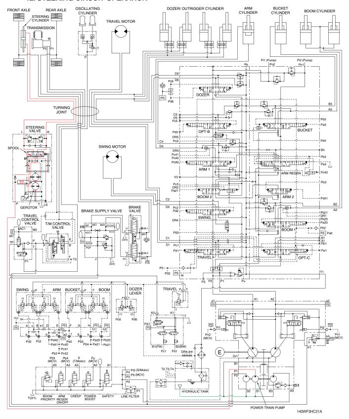
When the steering wheel is turned to the left or right, the spool within the steering valve turns left or right hand direction: Because the spool is connected with steering column.
