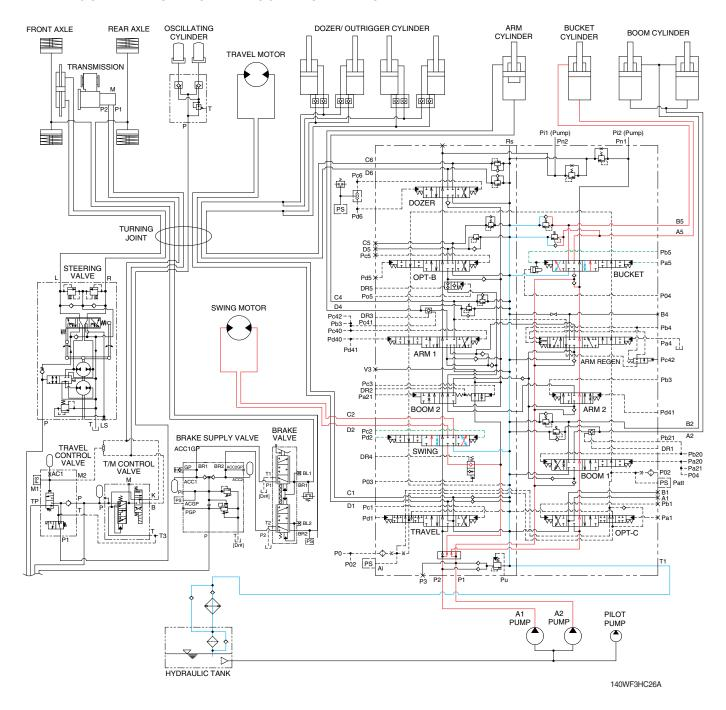
When the swing and bucket functions are operated, simultaneously the swing spool and bucket spool in the main control valve are moved to the functional position by the pilot oil pressure from the remote control valve.
