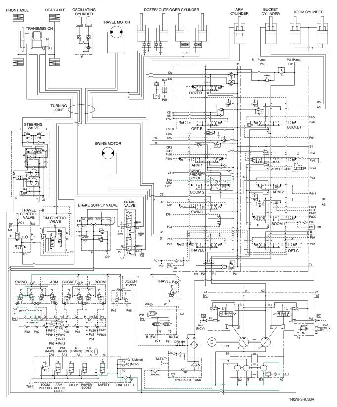
When carrying out the combined operation of swing and arm of the left control valve, the swing speed can be lowered than arm speed.
