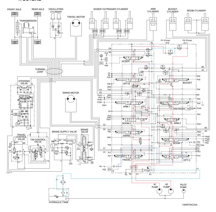
The oil from the A1 and A2 pump flows through the neutral oil passage, bypass oil passage and confluence oil passage in the main control valve. Then the oil goes to each actuator and operates them. Check valves and orifices are located on these oil passage in the main control valve. These control the oil from the main pumps so as to correspond to the operation of each actuator and smooth the combined operation.
