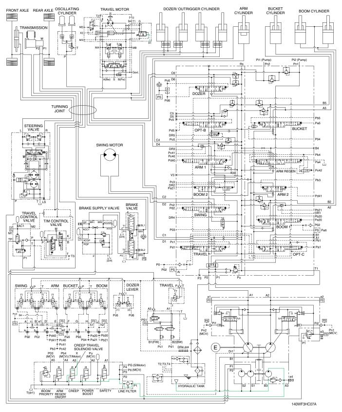
When the creep switch on the dashboard of the steering column is pushed ON, the creep travel solenoid valve is actuated.
