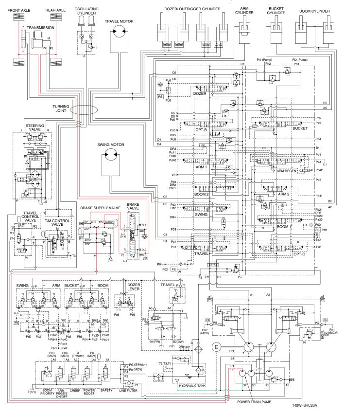
When the brake pedal (valve) is pushed, the discharged oil from the transmission pump (P2) flows into the front and rear axle brake disc through the brake supply valve.
