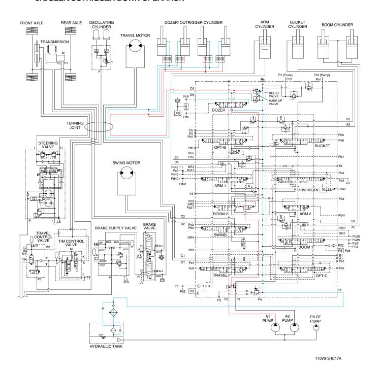
When the dozer control lever is pushed forward, the dozer spool in the main control valve is moved to the dozer down position by the pilot oil pressure from the remote control valve.
