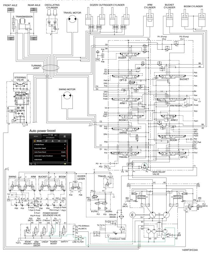
When the power boost switch on the left control lever is pushed ON, the power boost solenoid valve is actuated, the discharged oil from the pilot pump flows into **Pu** port of the main relief valve in main control valve; then the setting pressure of the main relief valve is raises from 350 kgf/cm² to 380 kgf/cm² for increasing the digging power. And even when press continuously, it is canceled after 8 seconds.
