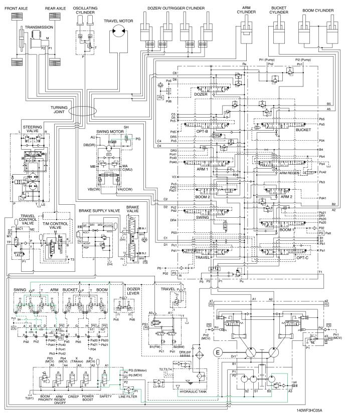
When the swing control lever or arm in control lever is tilted, the pilot oil flows into SH port through main control valve. This pressure move spool so, discharged oil from pilot pump flows into swing motor PG port. This pressure is applied to swing motor disc, thus the brake released.
