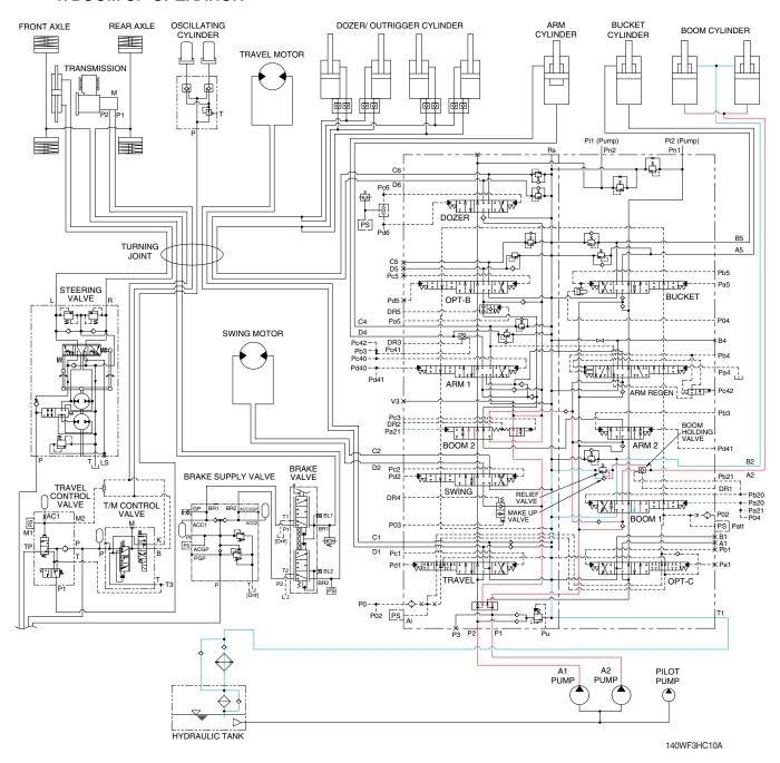
When the right control lever is pulled back, the boom spools in the main control valve are moved to the up position by the pilot oil pressure from the remote control valve.
