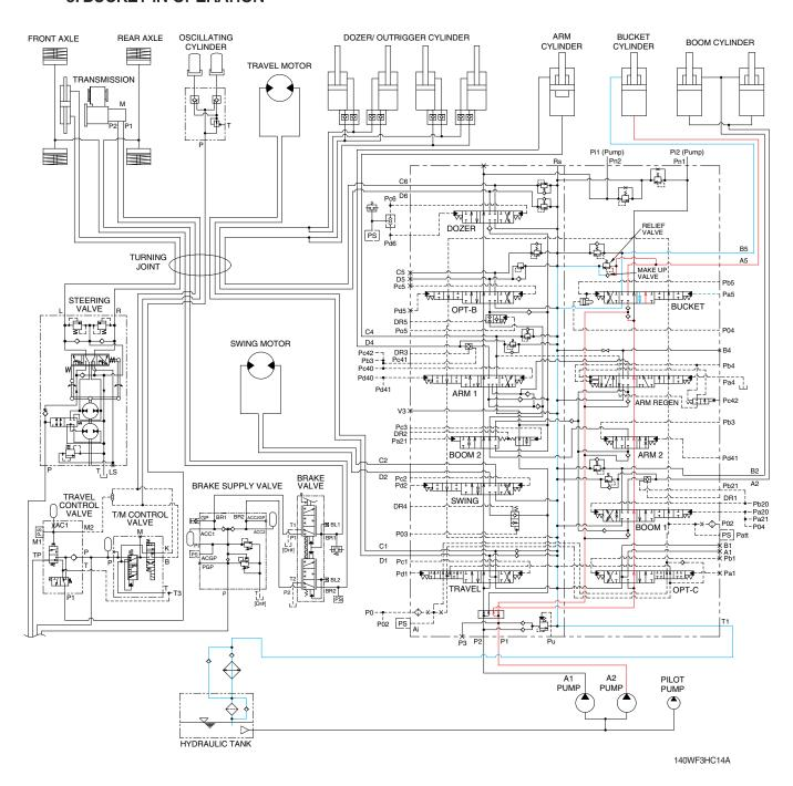
When the right control lever is pulled left, the bucket spool in the main control valve is moved to the roll in position by the pilot oil pressure from the remote control valve.
