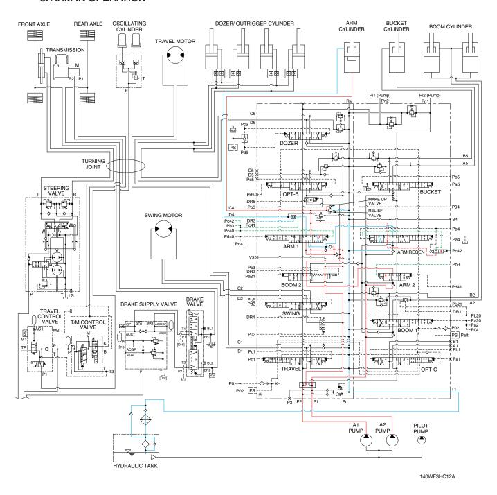
When the left control lever is pulled back, the arm spools in the main control valve are moved to the arm in position by the pilot oil pressure from the remote control valve.
