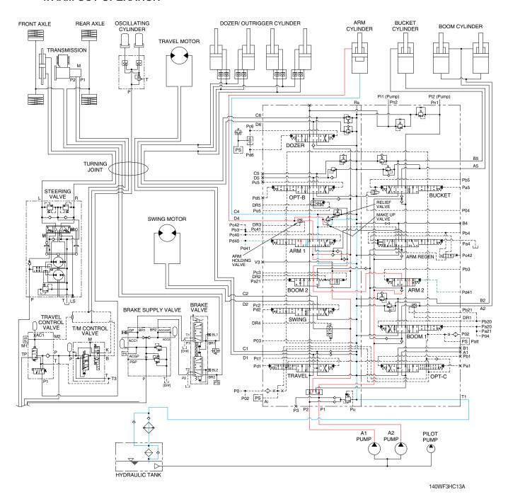
When the left control lever is pushed forward, the arm spools in the main control valve are moved to the arm out position by the pilot oil pressure from the remote control valve.
