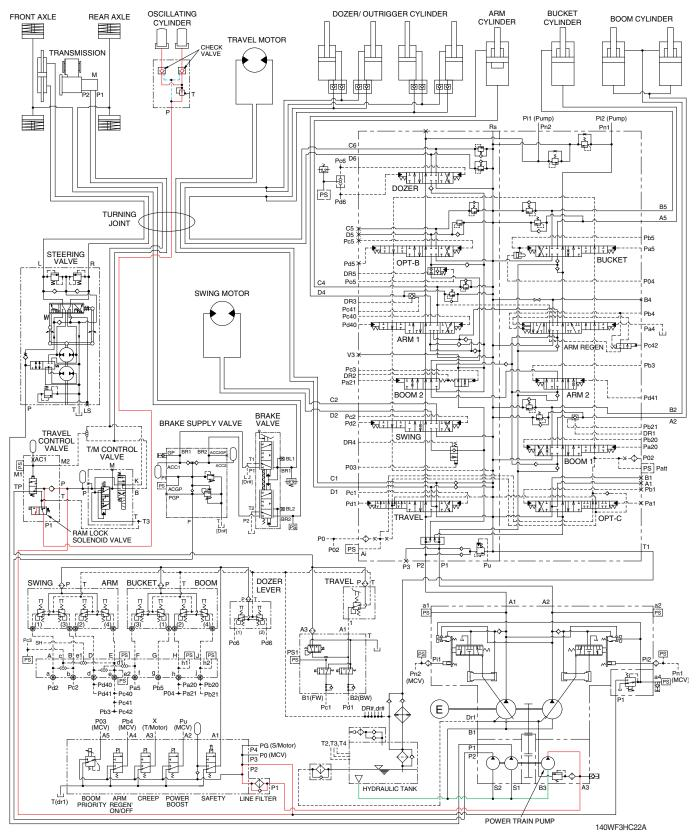
When the ram lock switch on the dashboard of the steering column is selected OFF position, the ram lock solenoid valve is changed over.
