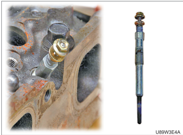
(1) Glow plug (2) Injector
