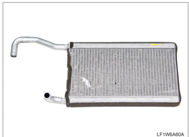
18. Unscrew the heater core fastener (1) to remove the heater core (2).
