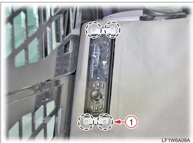
25. Unscrew 4 stereo mounting screws (1) and pull out the stereo assembly.
