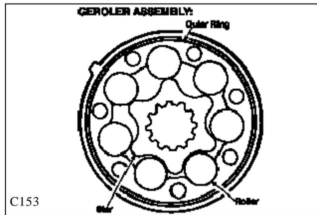
Because of the different number of teeth on the star and outer ring, the star rotates in an eccentric circular orbiting motion from the housing center line. ( fig. C154 )
