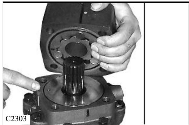
14 Inspect the gears and rollers for wear such as scratches and pitting. (fig. C2301, C2302) Replace worn parts as required. Do not mix the position of the rollers in the geroler section housing.
