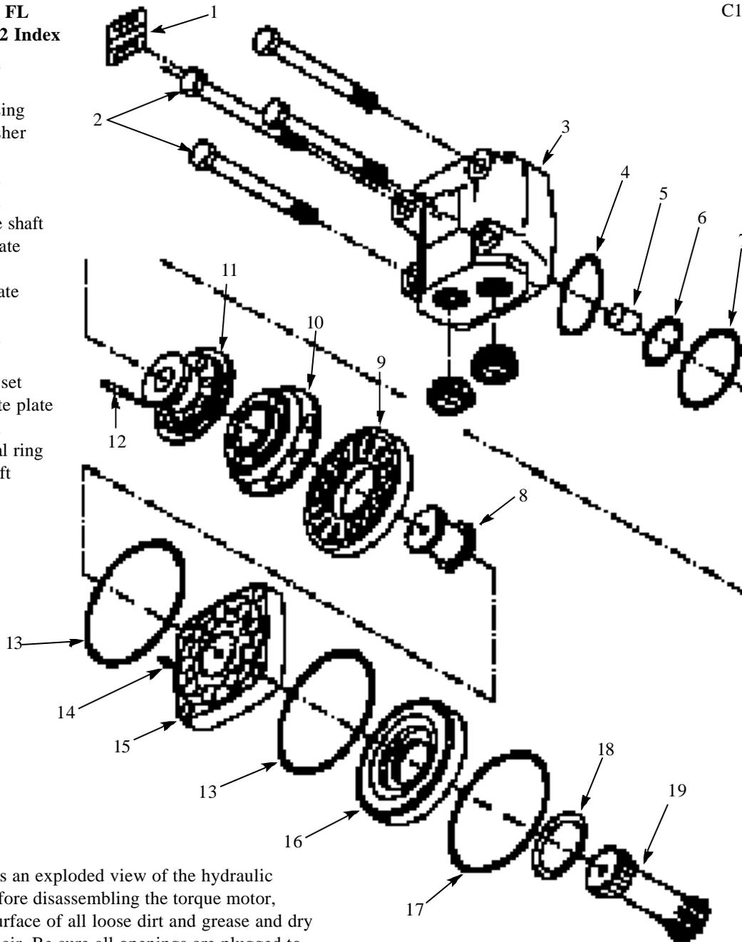
Fig. C1892 shows an exploded view of the hydraulic torque motor. Before disassembling the torque motor, clean the outer surface of all loose dirt and grease and dry with compressed air. Be sure all openings are plugged to prevent solvent or soap entering the torque motor.
