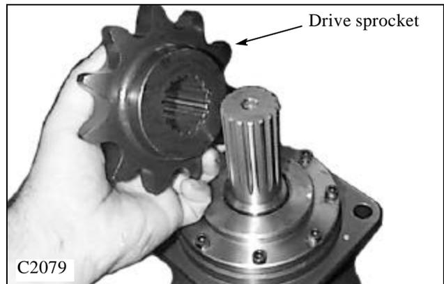
17 Install the sprocket, machined washer, lock washer and bolt. Apply Loctite 242 (blue) to the threads of the bolt before torquing (fig. C2080) and torque the bolt to 25 ft lbs. (34 Nm).
