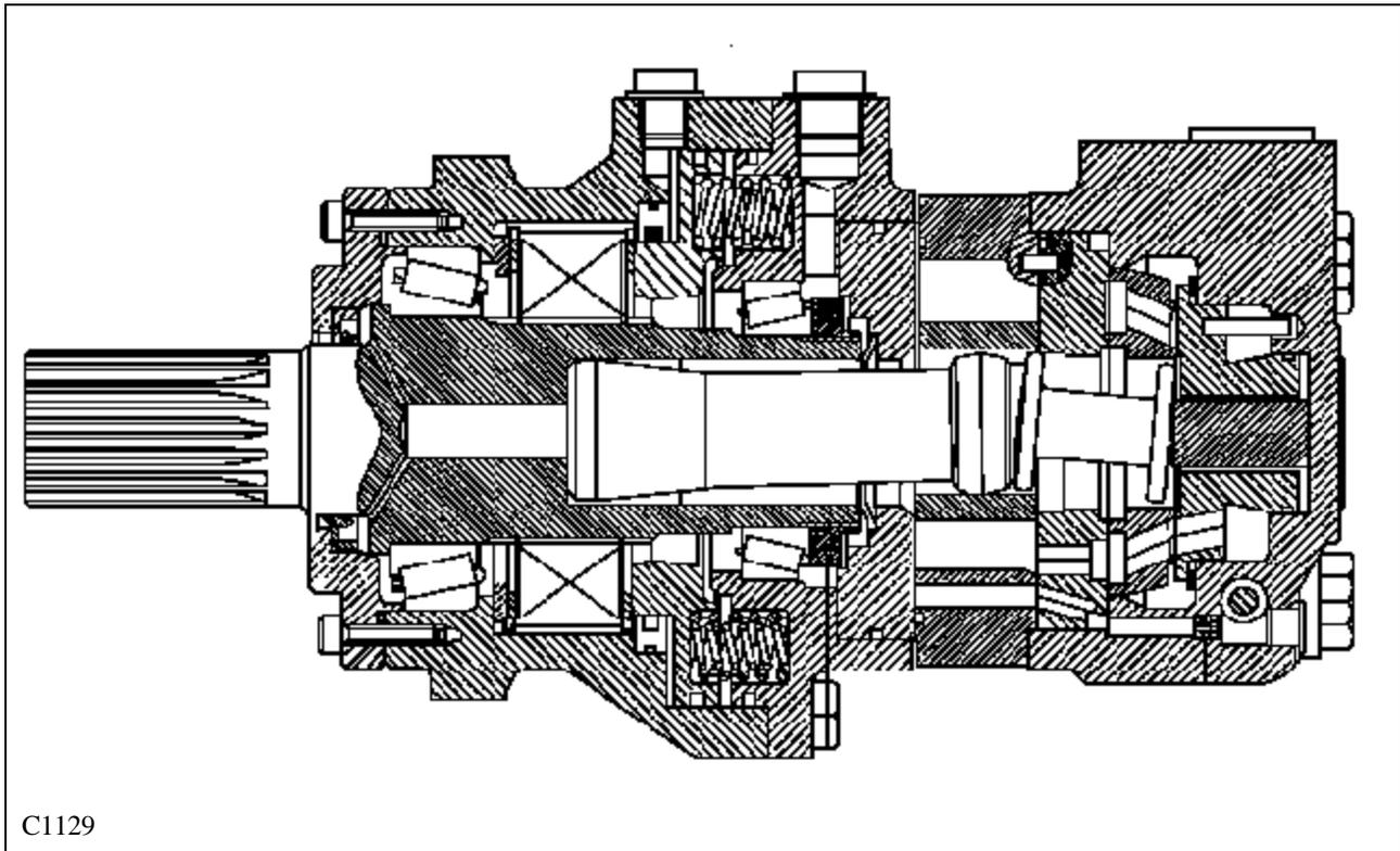
Fluid enters the housing through the inlet port and is directed to the balance plate. The balance ring contains an inner and outer seal to separate the high and low pressure fluid passages. Fluid passes through the stationary balance plate to the rotating disc valve. The rotating disc valve ports the fluid to the stationary valve plate and the proper side of the geroler pockets causing the rotor star to turn.
