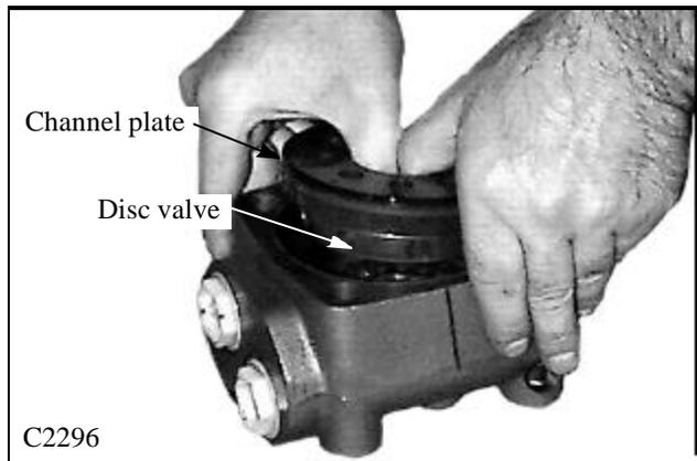
11 Remove the disc valve and balance plate from the valve housing section. (fig. C2297, C2298)
