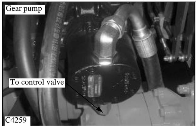
12 Connect the inlet fitting and hose to the auxiliary gear pump. (fig. C4259a) Torque the fittings and hoses to the specifications listed in the Torque Chart Section 2.13.
