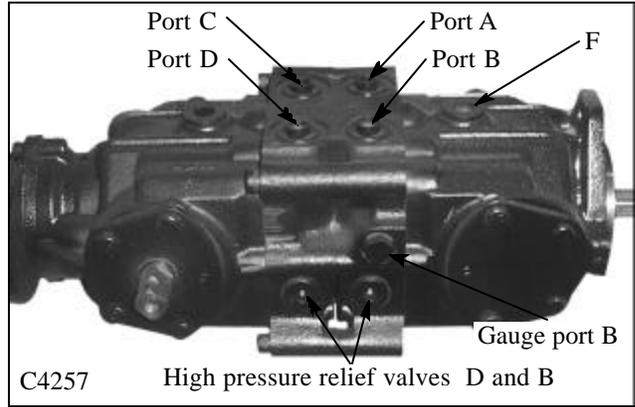
**NOTE:** Without Internal charge pump model shown
