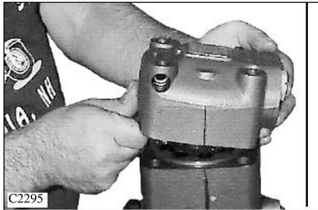
10 Remove the channel plate. (fig. C2296)
