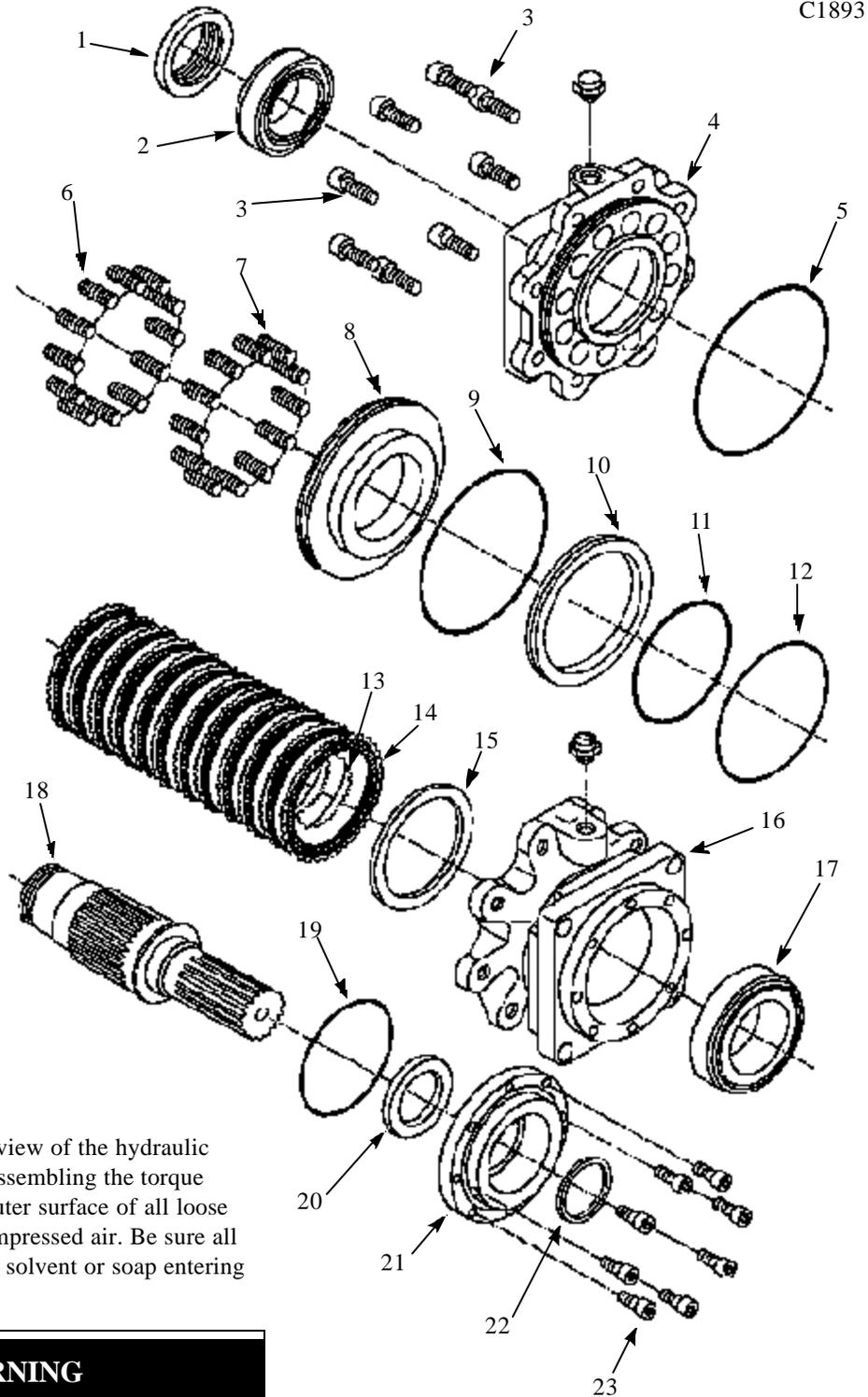
Fig. C1893 shows an exploded view of the hydraulic torque motor brake. Before disassembling the torque motor and or brake, clean the outer surface of all loose dirt and grease and dry with compressed air. Be sure all openings are plugged to prevent solvent or soap entering the torque motor.
