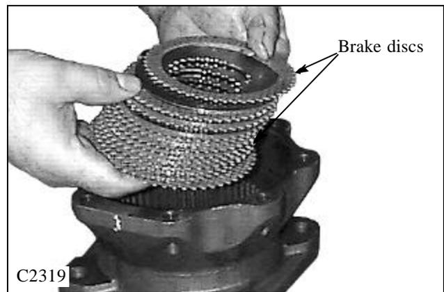
6 Install the piston to the housing, over the brake discs. (fig. C2318) Use new seals when assembling the motor. Align one of the piston spring pockets with the hydraulic inlet port opening in the housing. (fig. C2316)
