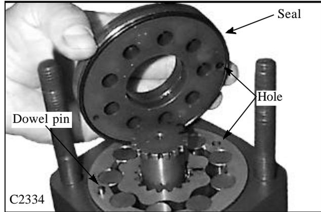
19 Install the disc valve to the valve drive. (fig. C2335) Align the mark on the valve drive with a hole in the outer rim.
