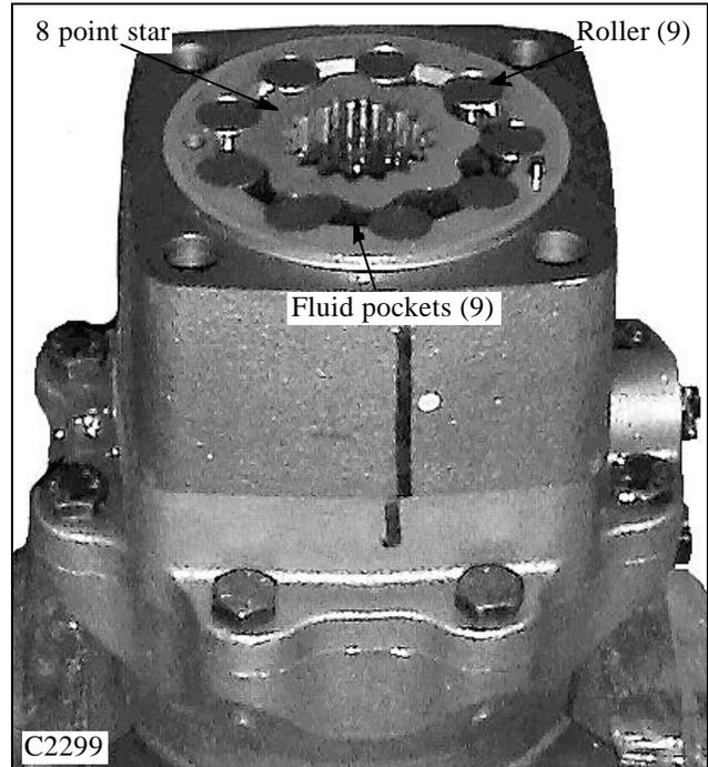
Example shown in fig. C166 is one complete star orbit, or one sixth of the output shaft rotation. The star must travel through 6 complete orbits for each single rotation of the output shaft creating a speed reduction of 6 to 1. The use of 7 fluid power pockets with the 6 to 1 ratio provides 42 fluid power cycles per each complete shaft revolution. **NOTE: Actual star point count is 8. This is only an example.**
