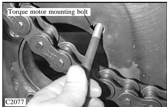
16 Remove the drive motor sprocket and bolt. Visually inspect the drive motor sprocket. Check for worn or damaged teeth on both the outside of the sprocket, and the inside spline (fig. C2079).
