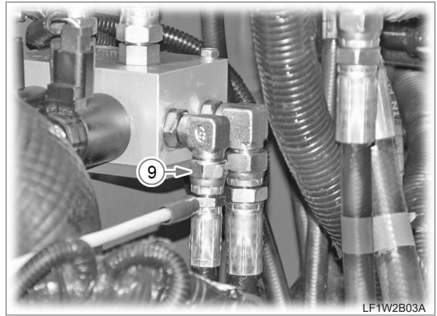
35. Connect the hydraulic hose (9) from the HST pump to the quick-attachment valve.
