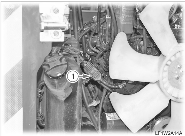
39. Disconnect the engine wiring connector (1) from the front left side of the engine.
