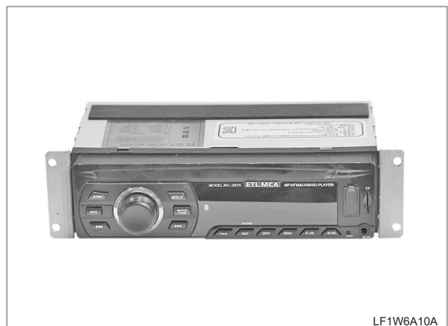
26. Disconnect the stereo wiring connector (1) and antenna cable (2) to remove the stereo (3).
