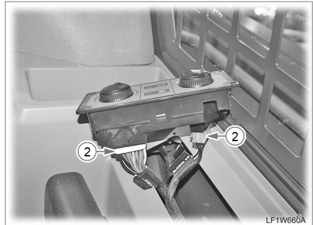
13. Disconnect the A/C controller wiring connector (2).
