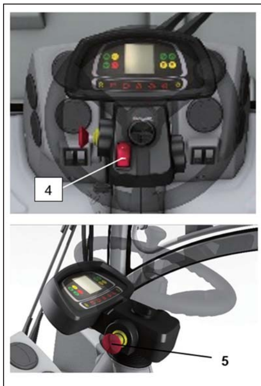
Fig. 34 Control elements on the steering column
