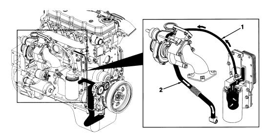
(1) Lubrication for the turbocharger
