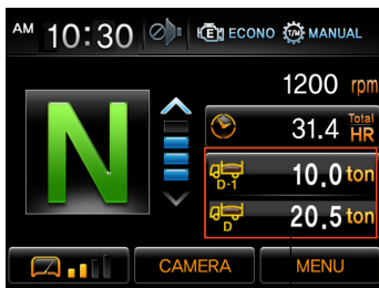
The example of the weighing system
