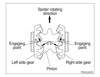
② When traveling on soft ground (Resistance from road surface to left and right tires is different)
