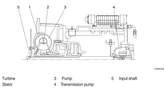
The converter is working according to the Trilok-system, i.e. it assumes at high turbine speed the characteristics, and with it the favorable efficiency of a fluid clutch.
