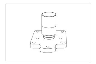
(6) Secure mounting flange(1) with cap screws(70) and tighten to half torque and then full torque in a diagonal sequence to figure as per assembly drawing.
