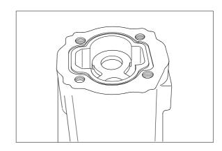
Side wear plate(35) complete with seal and back up seal down through the housing to the bottom of the gear pockets.
