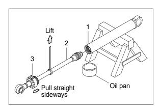
Note that the plated surface of piston rod(2) is to be lifted. For this reason, do not use a wire sling and others that may damage it, but use a strong cloth belt or a rope.
