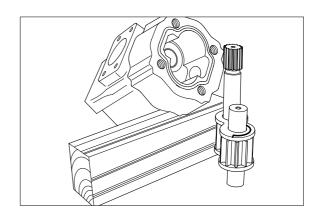
\*\* Mark the gears using a soft pencil or felttip pen to ensure reassembly in the same relative position, then withdraw the drive shaft/gear and driven gear separately to prevent jamming.
