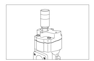
(5) Apply a small ring of loctite low strength gasket eliminator to the interface of mounting flange(1) and fit to front cover(2), ensure that location sleeve(85) is in place and correctly positioned.
