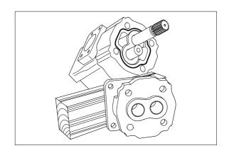
(4) Before removing wear plate(30) from the body(9) mark it using a soft pencil or a felt-tip pen to ensure correct reassembly. Remove wear plate(30) complete with wear plate seal and back up seal.
