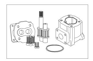
(2) Place body(9) vertically with front section gear pockets upper most.
