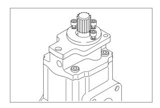
(2) Remove the cap screws(80) securing the cover(2) to body(9).
