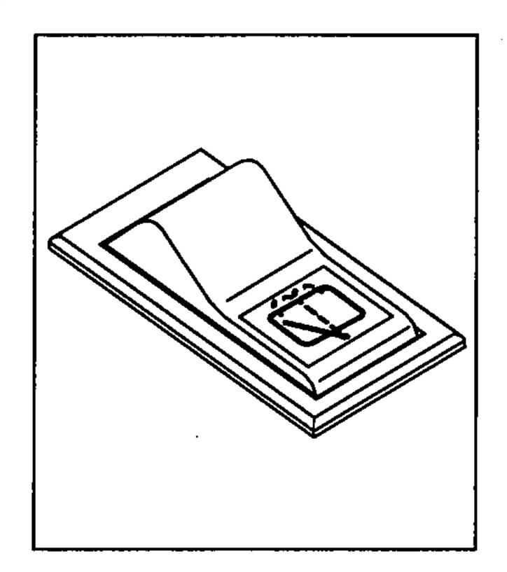
(1) The switch use to operates the rear wiper and washer by two step.
