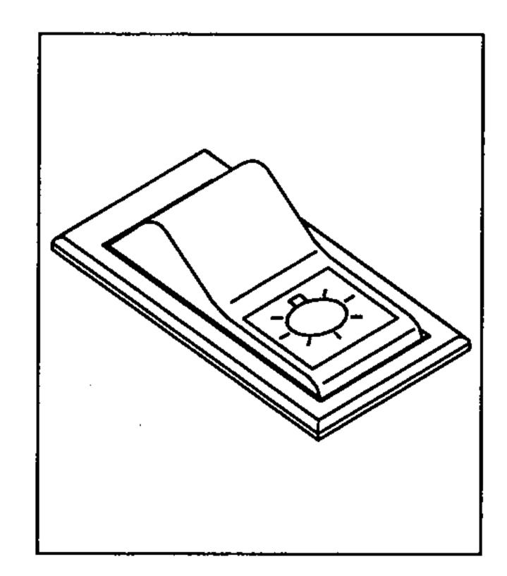
(1) This switch use to operates the clearance lamp and head light by two step.
