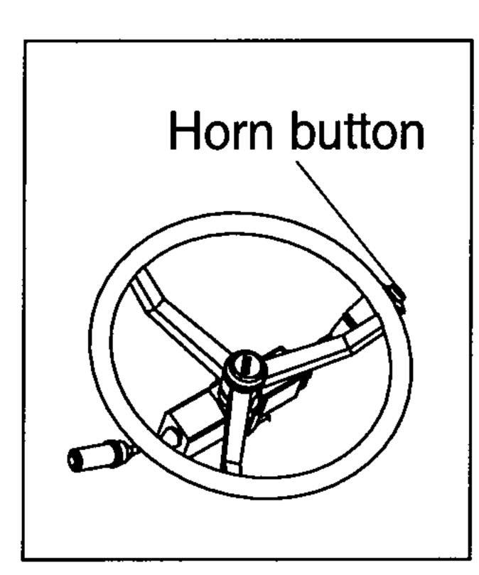
(1) If you press the button on the top of the multifunction switch, the horn will sound.
