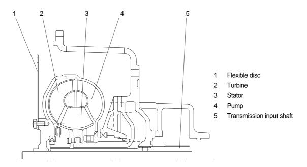
The converter is working according to the trilok-system, i.e. the converter assumes at high turbine speeds, the characteristics and therefore the favorable efficiency of a hydraulic clutch. The converter is designed according to the engine output, so that the most favorable operating conditions for each installation purpose are obtained.
