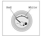
(1)This gauge indicates the amount of fuel in the fuel tank
