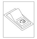
(1)This switch is used for starting the engine in cold weather. If pressed, starting aid fluid is injected for easier engine
