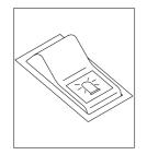
(1)This switch turns ON the rotary light on the cab.
