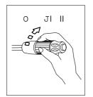
When the switch Jiposinion, the wiper moves intermittent
