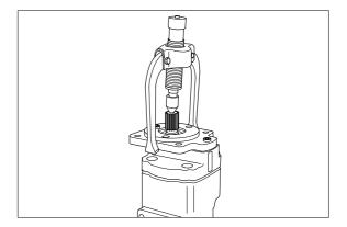
Remove the shaft seal(55) from cover(2) making sure that no damage is sustained to the surface of the seal bore in the cover.
