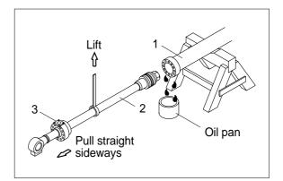
Note that the plated surface of piston rod(2) is to be lifted. For this reason, do not use a wire sling and others that may damage it, but use a strong cloth belt or a rope.
