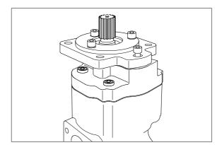
Fit the gears within the housing taking care of replace as marked, with the teeth reassembled to the original related position.
