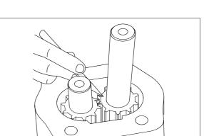
(6) Remove wear plate complete with wear plate seal and back up seal. Mark the gears using a soft pencil or felt-up pen to ensure reassembly in the same relative position.
