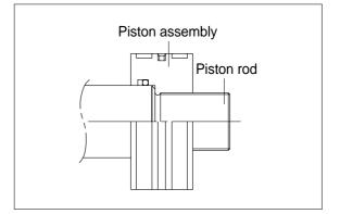
(5) Tighten piston nut(17) and screw(18) to piston rod(2)
