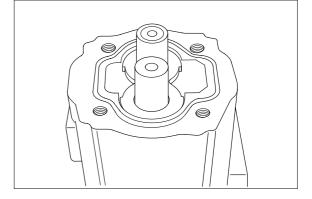
(8) Fit new interface seal(61) into groove in body(4).
