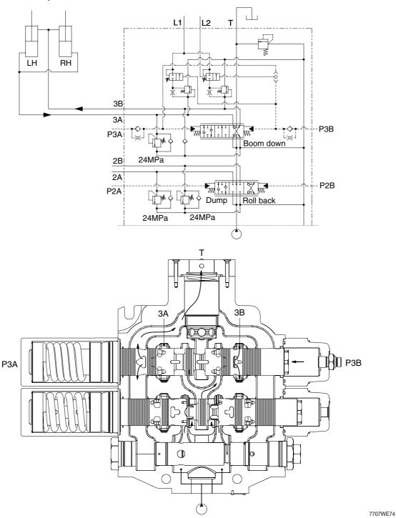
When the pilot pressure from remote control valve is supplied to the pilot port(P3B), the spool moves to the left and the neutral passage is closed.
