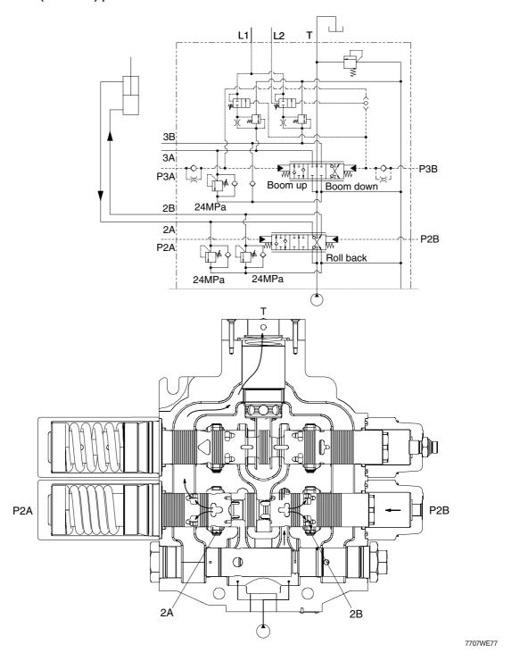
When the pilot pressure from remote control valve is supplied to the pilot port(P2B), the spool moves to the left and the neutral passage is closed.
