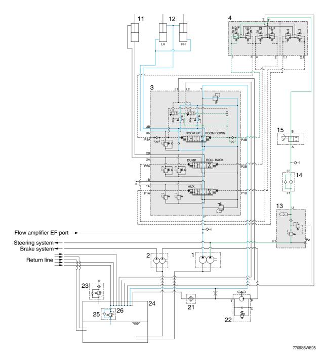
Float is achieved by opening 2 large capacity check valves(A) fitted into the bolt on float check block. These check valves connect each of the boom service ports(3A, 3B) to the tank gallery. Opening of these valves is controlled by pilot pressure from the hydraulic pilot control valve(4).
