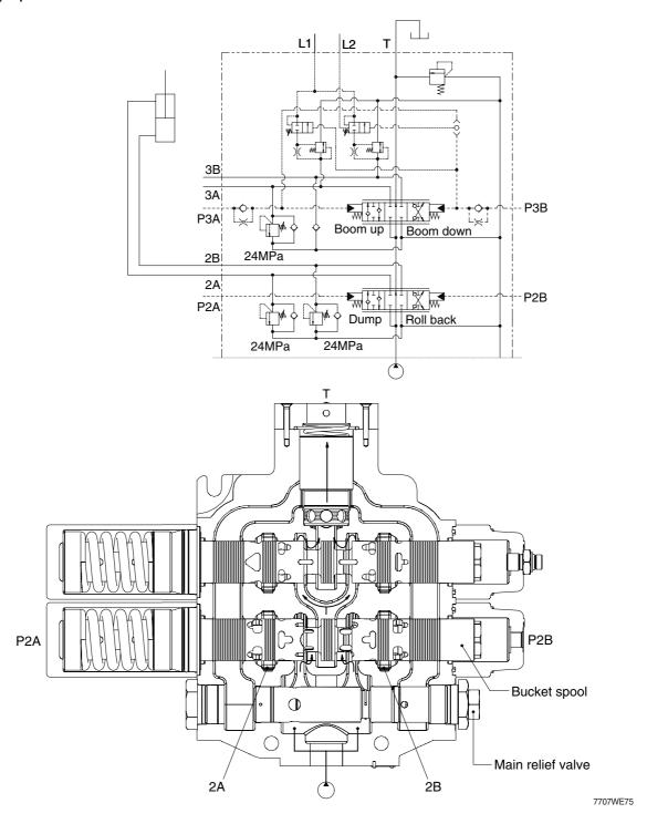
If the remote control valve is not operated, the oil supplied from the pump port passage through the neutral passage to the low pressure passage at the outlet section, and then return to the tank port.
