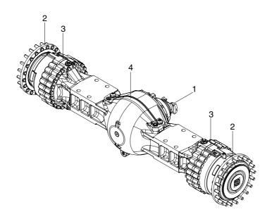
1 Input 2 Output 3 Brake 4 Axle housing
