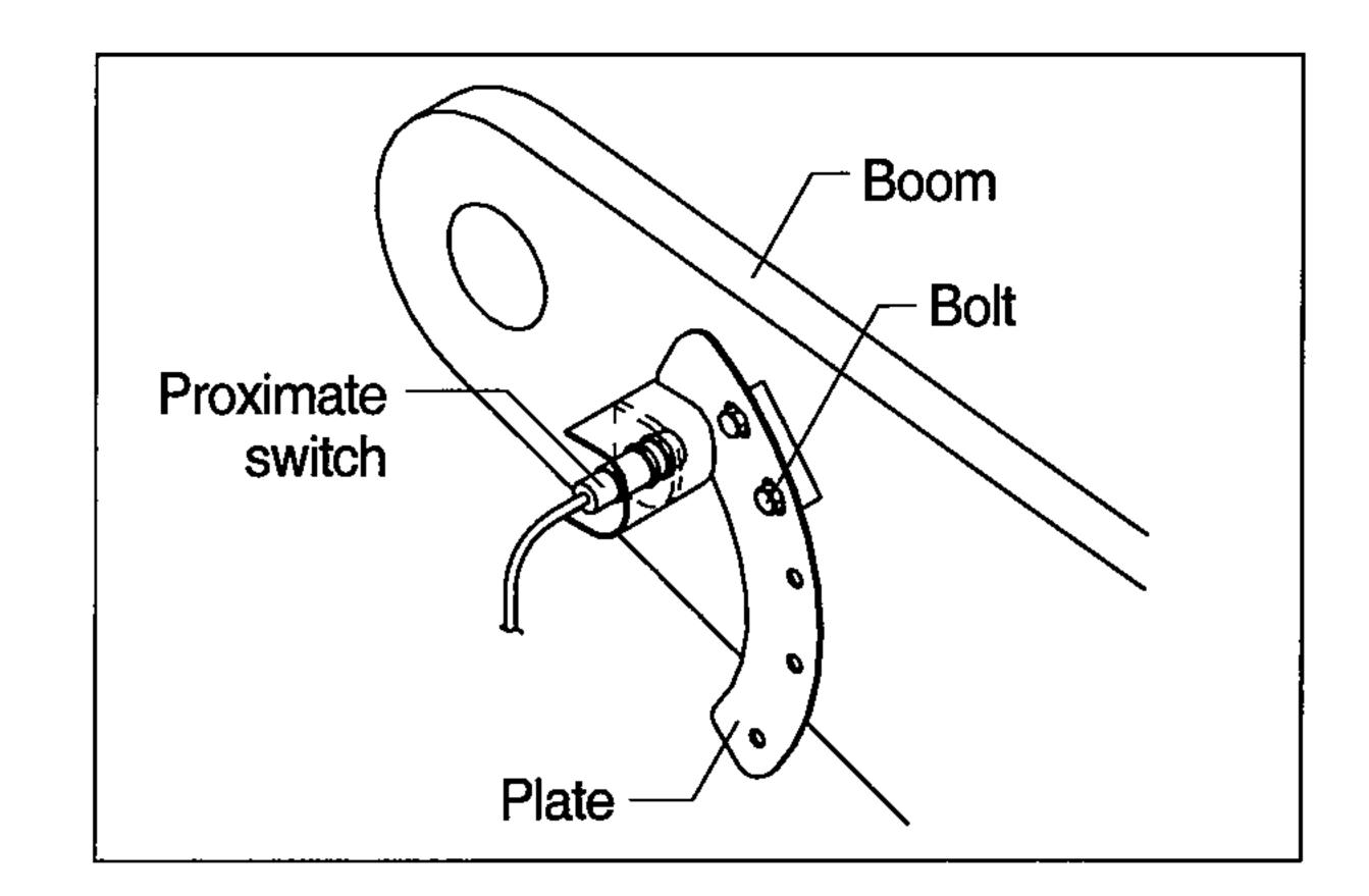
2) Loosen bolts then tighten them after adjusting the plate so that it comes in contact with the center of the probe of the proximate switch.
