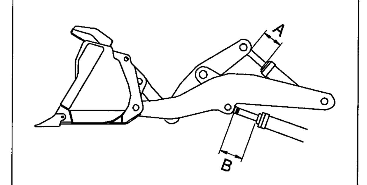
A: Retraction of bucket cylinder rodB: Retraction of boom cylinder rod
