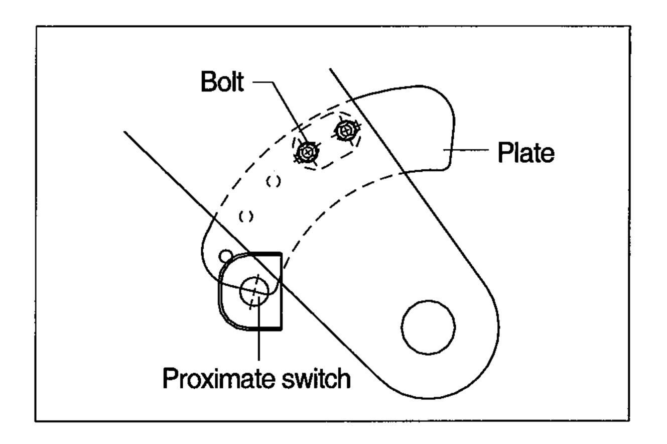
3) Loosen the nuts so that a clearance between the plate and the probe of the proximate switch are 3±1mm.
