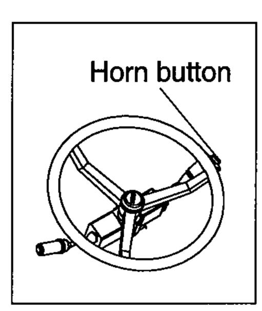
(1) If you press the button on the top of the multifunction switch, the horn will sound.
