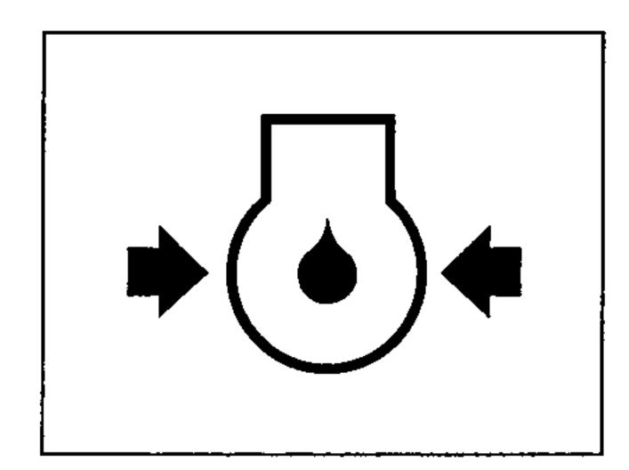
(1) If lamp comes ON during engine operation, shut OFF engine immediately. Check oil level.
