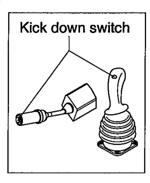
(1) The kick-down switch into first gear is not allowed. Press the switch and release the switch. The transmission downshifts one gear speed, provided that an engine overspeed would not occur.
