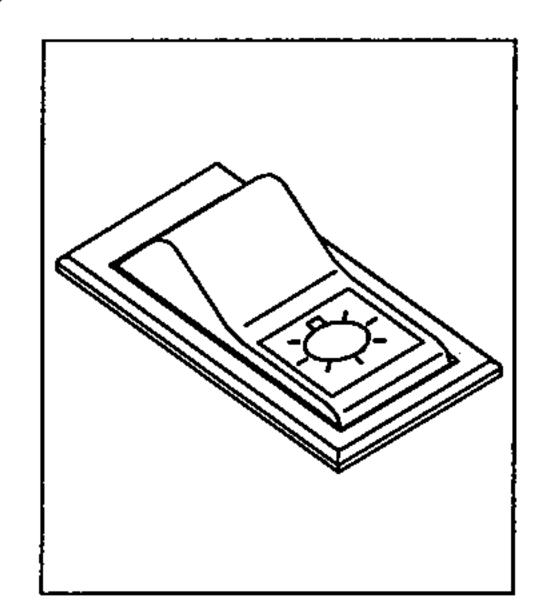
(1) This switch use to operates the clearance lamp and head light by two step.
