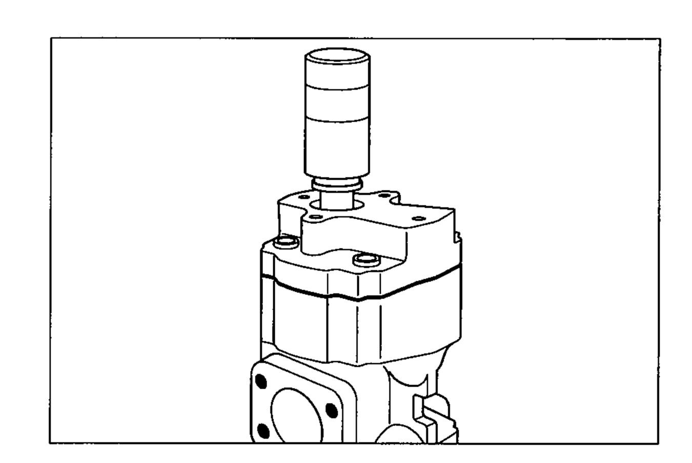
(5) Apply a small ring of loctite low strength gasket eliminator to the interface of mounting flange(1) and fit to front cover(2), ensure that location sleeve(85) is in place and correctly positioned.
