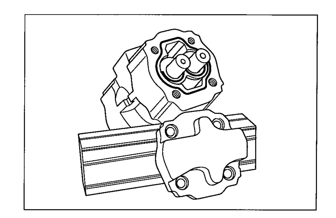
Again to ensure correct reassembly mark remaining wear plaet(35) using a soft pencil or a felt-tip pen.
