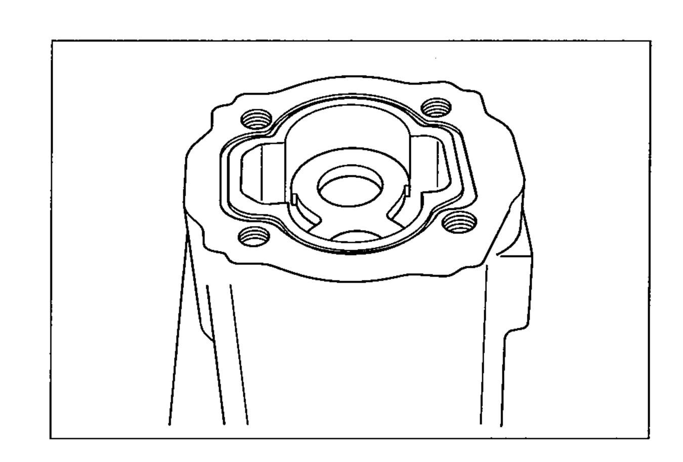
Side wear plate(30) complete with seal and back up seal down through the housing to the bottom of the gear pockets.
