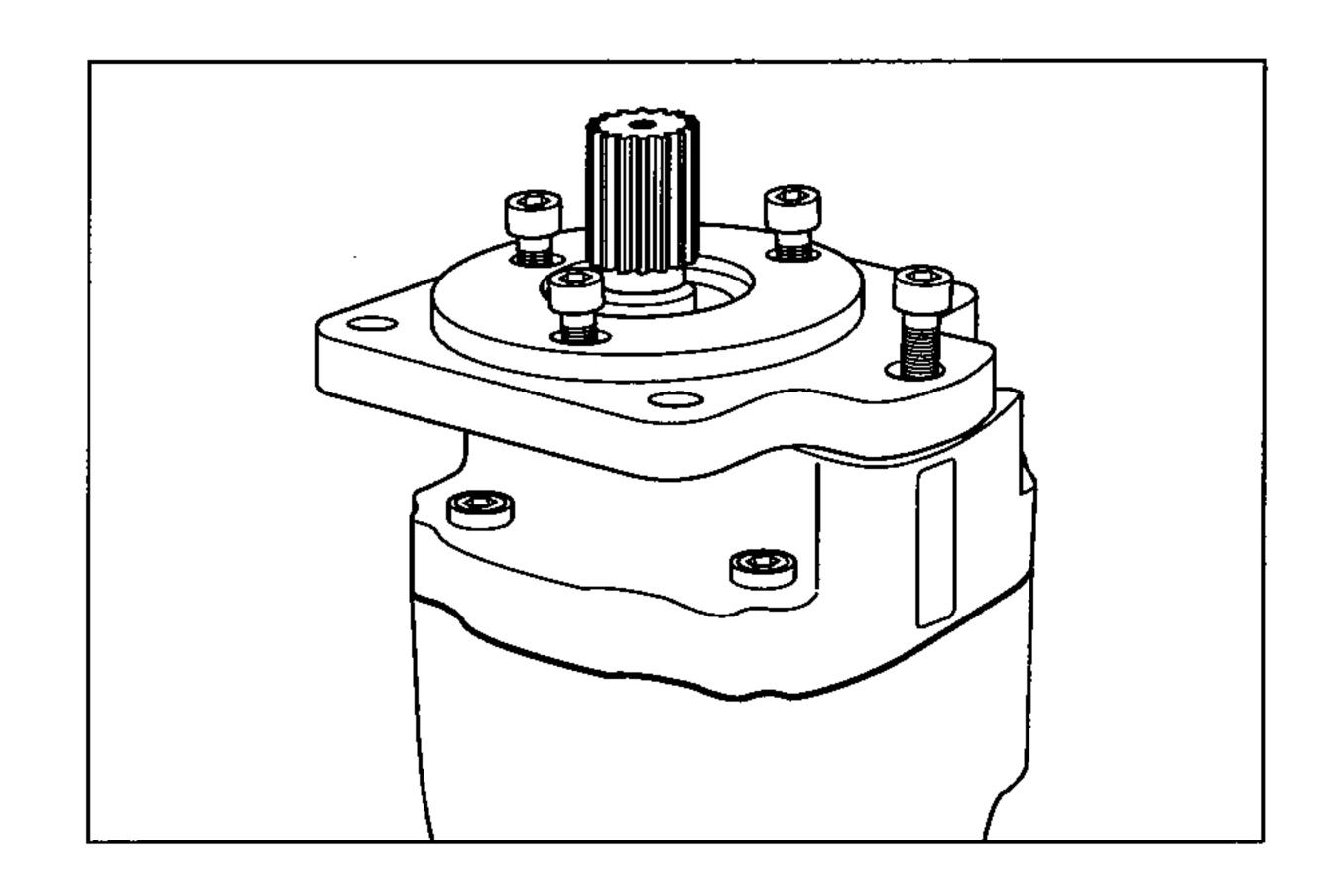
(2) Remove the cap screws(80) securing the cover(2) to body(4).
