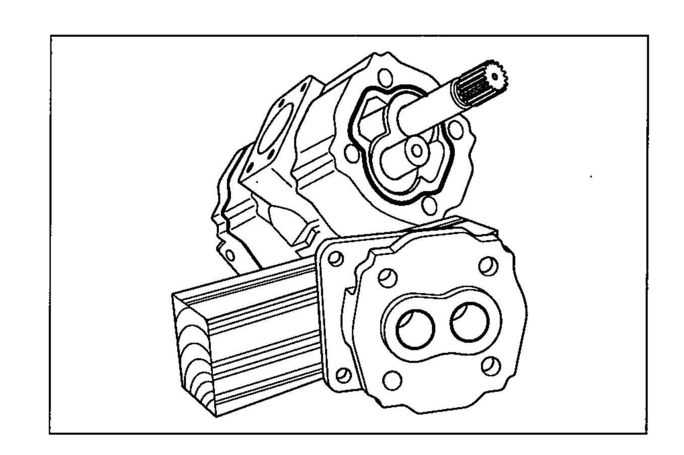
(4) Before removing wear plate(35) from the body(4) mark it using a soft pencil or a felt-tip pen to ensure correct reassembly. Remove wear plate(35) complete with wear plate seal and back up seal.
