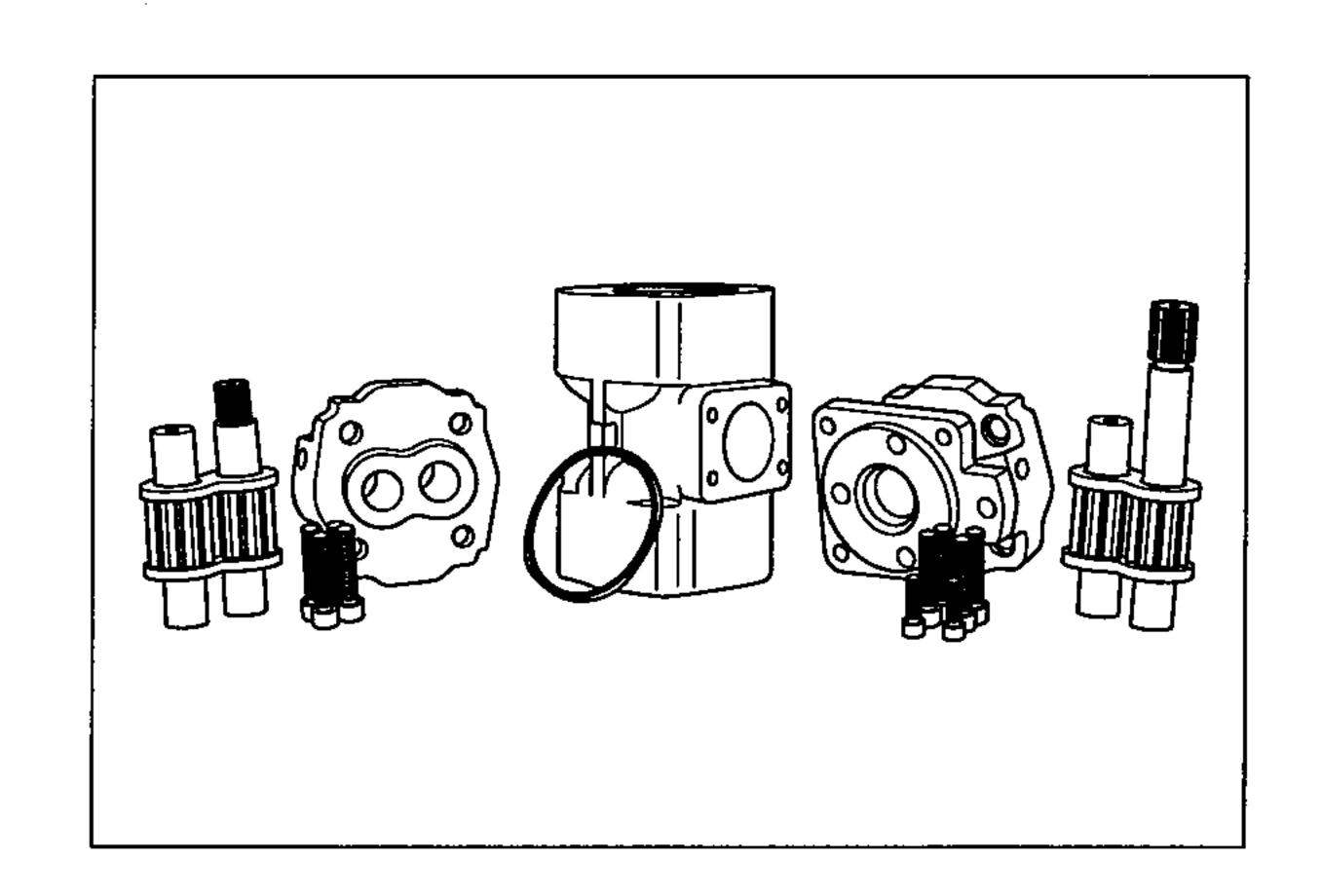
(2) Place body(4) vertically with front section gear pockets upper most.
