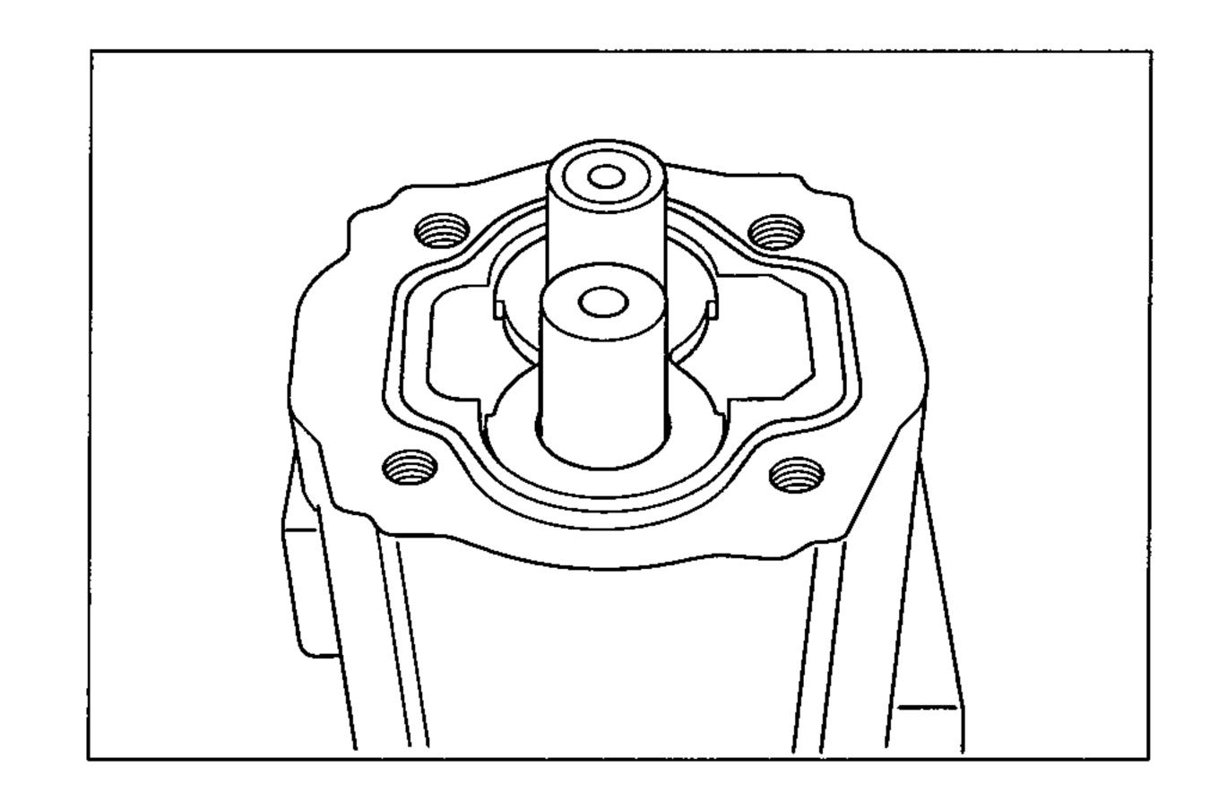
(8) Fit new interface seal(61) into groove in body(4).
