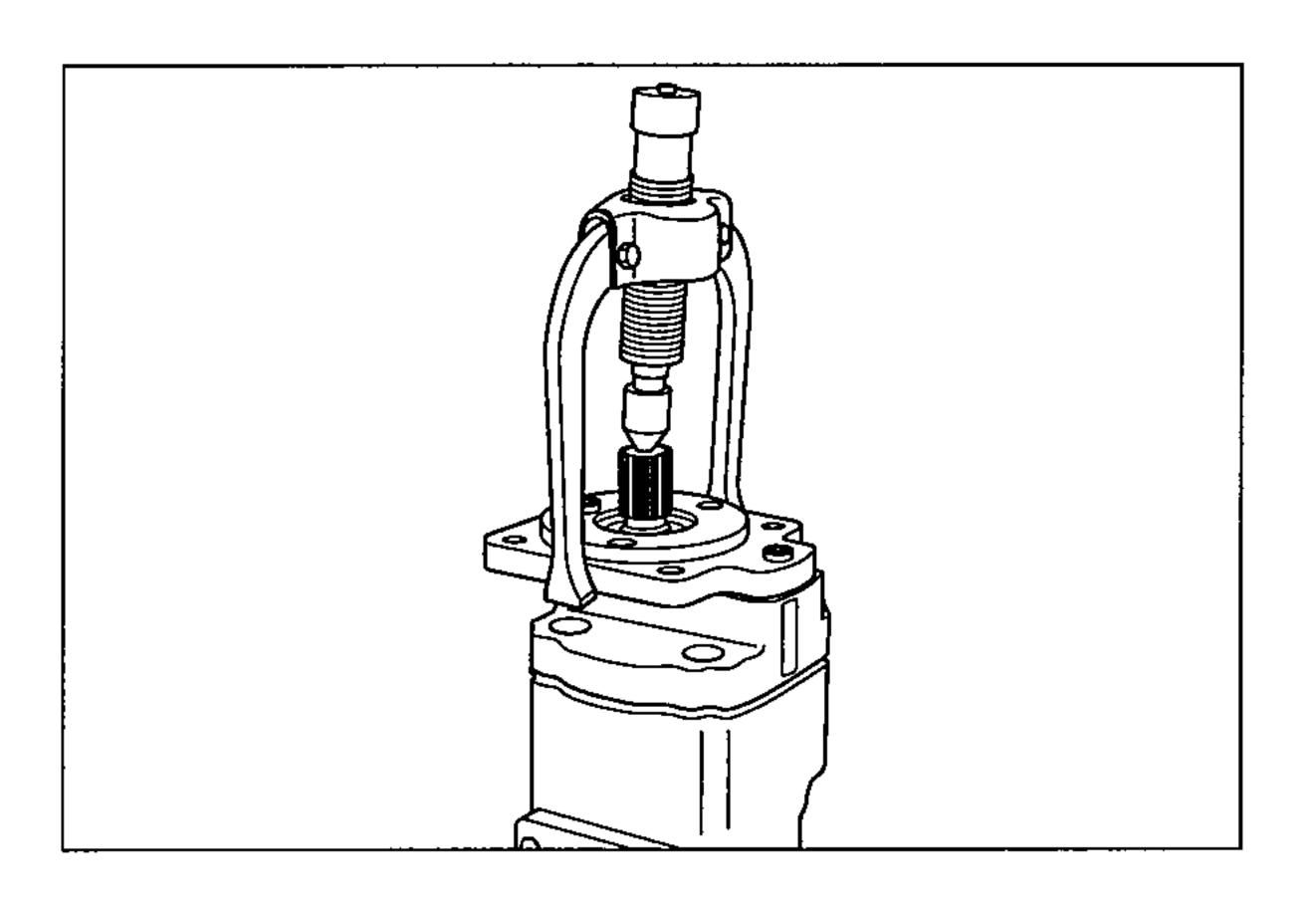
Remove the shaft seal(55) from cover(2) making sure that no damage is sustained to the surface of the seal bore in the cover.
