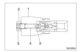
(2) Loosen hex nut(2), and remove adjust screw(3), spring(4) and pilot poppet(5).
