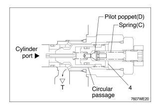
As oil flows from the cylinder port to the tank passage through the orifice(2) of the piston(A), the pressure of the chamber(3) comes to lower than that of the cylinder port. Then the piston(A) is lifted and seated to the pilot poppet(D).
