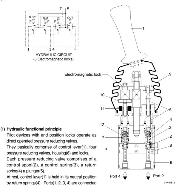
When control lever(1) is deflected, plunger(5) is pressed against return spring(4) and control spring(3).
