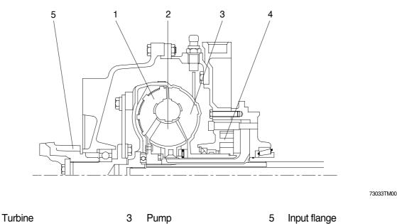
2 Stator 4 Transmission pump
