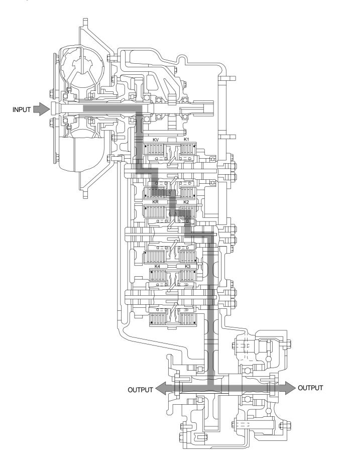
With the transmission in second forward, the forward clutch and second speed clutch are engaged.
