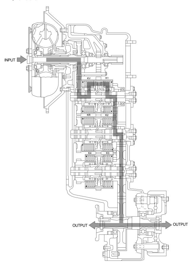
With the transmission in first forward, the forward clutch and the first speed clutch are engaged. The torque converter supplies torque to the drive gear which meshes with the gear on the forward clutch hub.
