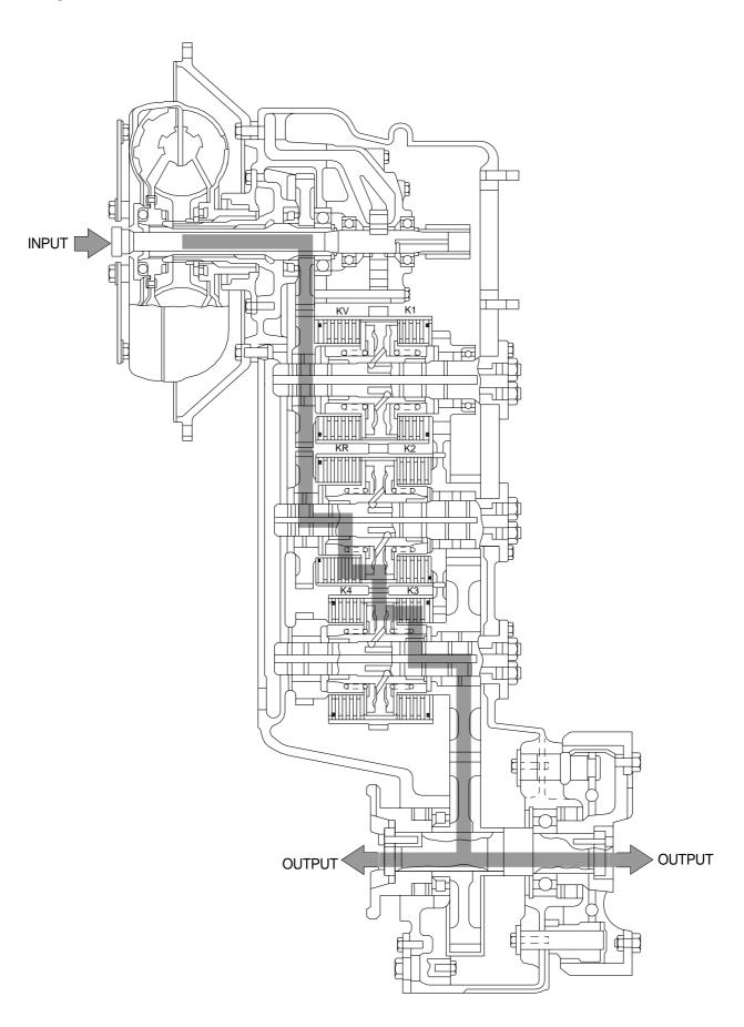
With the transmission in third speed reverse, the reverse clutch and third speed clutch are engaged. The torque converter supplies torque through the drive gear which meshes with the reverse gear hub.
