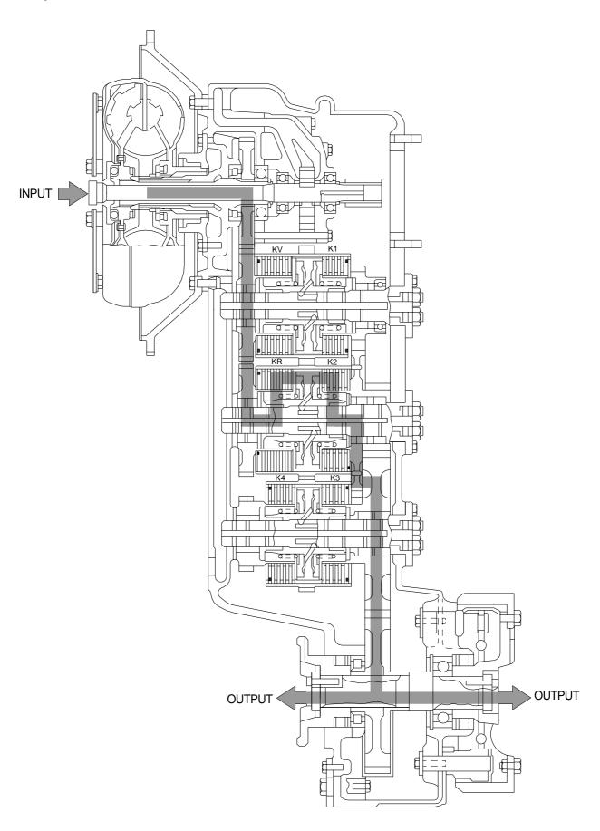
With the transmission in second gear reverse, the reverse clutch and second speed clutch are engaged. The torque converter supplies torque to the drive gear which meshes with the reverse clutch hub.
