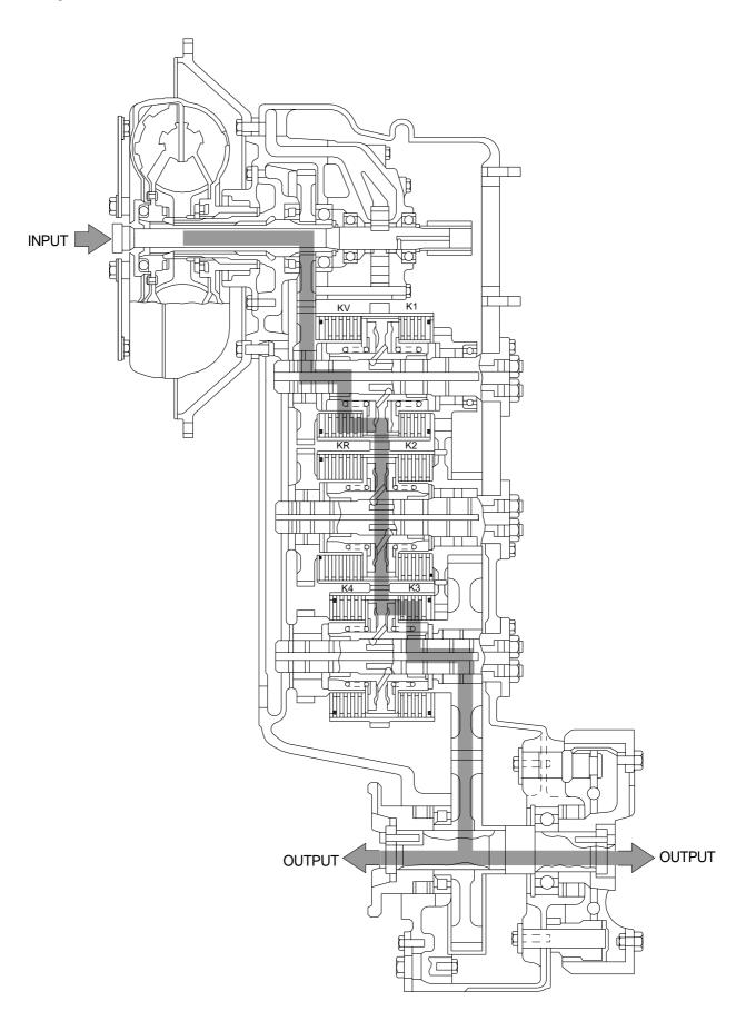
With the transmission in third forward, the forward clutch and third speed clutch are engaged. The torque converter supplies torque to the drive gear which meshes with a gear on the forward clutch hub.
