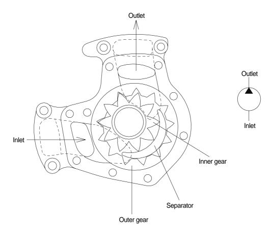
The transmission pump is a fixed displacement, internal gear type pump. The transmission pump is driven at engine speed off the impeller drive from the torque converter.
