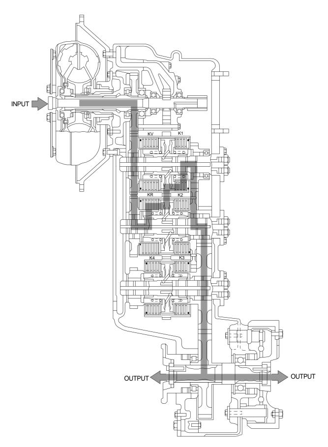
With the transmission in first gear reverse, the reverse clutch and first speed clutch are engaged. The torque converter supplies torque to the drive gear. The drive gear meshes with the gear on the reverse clutch hub.
