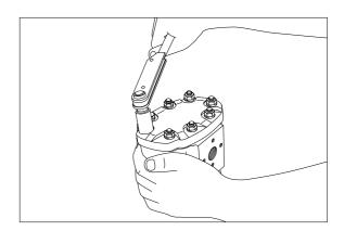
(2) Remove the rear cover(12) and stud bolt (29).
