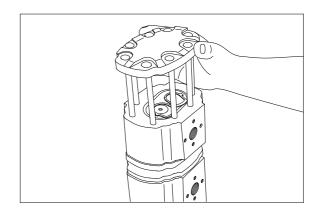
(3) Remove rear body(8) and spacer plate (15).
