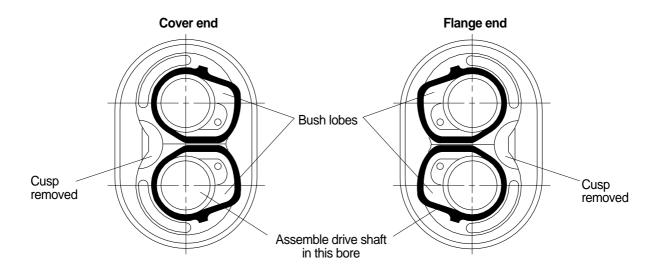
\* In the bushes are always assembled in the body with the C shape mating with the cusp removal flat the body.
