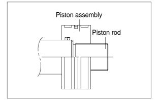
(5) Tighten piston nut(16) and screw(17) to piston rod(2)
