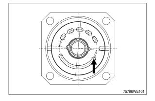
(10) Fit connection plate and control valve.
