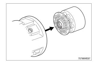
(6) Remove swash plate and bearing shells.
