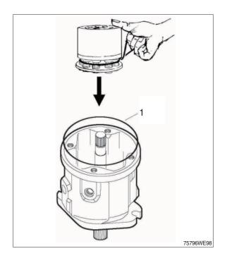
(7) Fit bearing (1) in connection plate.
