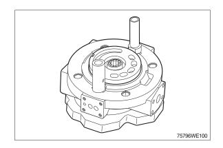
(9) For clockwise rotation pumps the distributor plate is off-set by 4° to the right from the centre position.
