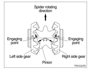
② When traveling on soft ground (Resistance from road surface to left and right tires is different)
