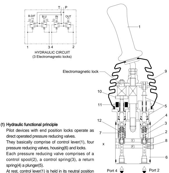
by return springs(4). Ports(1, 2, 3, 4) are connected to tank port T via drilling(8).
