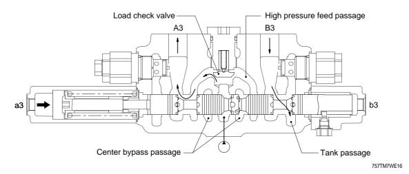
When the pilot pressure is led to the port(a3), the boom plunger is switched, and shut off center bypass passage.
