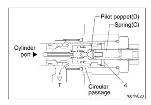
As oil flows from the cylinder port to the tank passage through the orifice(2) of the piston(A), the pressure of the chamber(3) comes to lower than that of the cylinder port. Then the piston(A) is lifted and seated to the pilot poppet(D).
