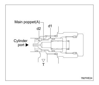
(2) When the cylinder port pressure comes to lower than the tank passage pressure (closer to negative pressure), the poppet (A) opens receiving the tank passage pressure for the difference in area between d2 and d1. Oil from the tank passage flows to the cylinder port in order to prevent cavitation.
