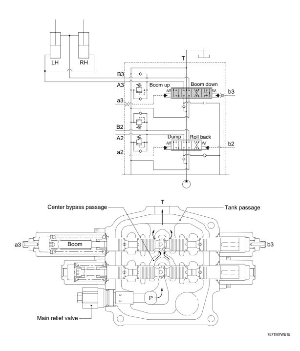
When the boom plunger is in neutral position, oil from the pump flows to the tank through the center bypass line.
