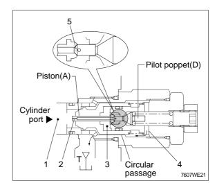
Oil from the cylinder port flows to the tank passage. As the pressure of the chamber(3) comes to lower still more, the main poppet(B) is lifted and pressured oil flows into the tank possage.
