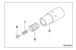
Do not disassemble pilot seat, because the pilot seat is assembled with pressure.
