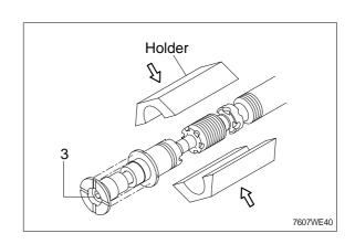
(4) Remove the plunger cap(3), spring guide (4), spring(5) and sleeve(6).
