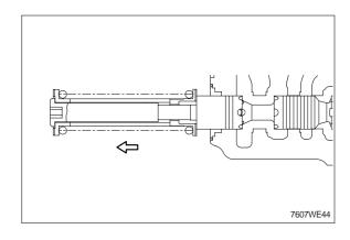
(3) Set the spool between holders and loosen plunger cap(3) by using vise.
