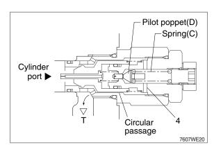
② As oil flows from the cylinder port to the tank passage through the orifice (2) of the piston (A), the pressure of the chamber (3) comes to lower than that of the cylinder port. Then the piston(A) is lifted and seated to the pilot poppet (D). Oil from the cylinder port flows to the tank passage through the orifice (5) of the pilot poppet (D), side hole (4) and the circular passage.
