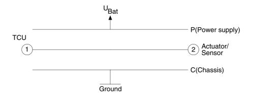
Open circuit  $R_{12} = R_{1P} = R_{1C} = R_{2P} = R_{2C} =$
