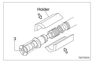
(4) Remove the plunger cap(3), spring guide(4), spring(5) and sleeve(6).
