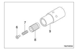
Do not disassemble pilot seat, because the pilot seat is assembled with pressure.
