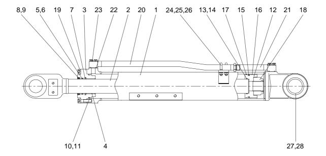
1 Tube assy 11 Back up ring 21 Pipe assy 2 Rod assy 12 **Piston** 22 O-ring 3 Gland Bolt 13 O-ring 23 4 Bushing 14 Back up ring 24 U-bolt 5 25 Rod seal 15 Piston seal Nut Spring washer 6 Back up ring 16 Wear ring 26 7 Buffer ring 17 **Dust ring** 27 **Bushing** 8 **Dust wiper** 18 Nut 28 **Dust seal** 9 Snap ring 19 **Bolt** 10 O-ring 20 Pipe assy
