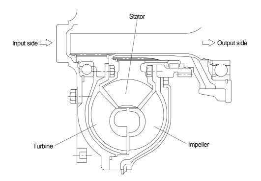
Torque converter is a stemless transmitting system to transmit engine power by means of hydraulic force. As usual, this system(torque converter) is consisting of three elements(impeller wheel, turbine wheel, stator wheel).... the impeller wheel connected to input shaft, the turbine wheel connected to output shaft and the stator wheel(guide bland) fixed to the housing.
