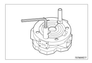
(14) Disassemble the guide of the opposite piston.
