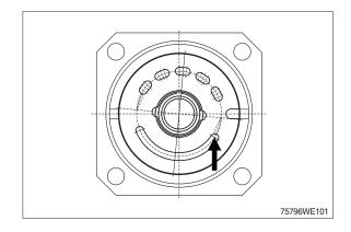
(10) Fit connection plate and control valve.
