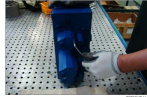
② Remove the cover, spring retainer, spring and spool.
