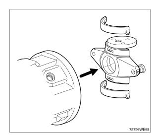
(7) Remove the circlip and the shaft seal.
