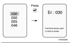
To go out from fault explanation window, press (a) button.
