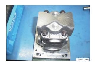
(14) Use air impact to assemble nuts.
