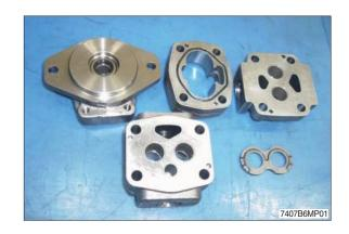
(2) Put section sub assembly on the assembly table. Assemble dowel pins.
