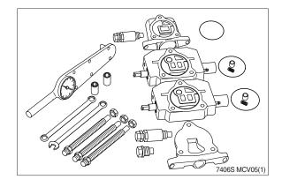
(2) Assemble tie rod nuts to one end of each tie rod with one or two threads showing. Insert tie rods through tie rod holes of inlet (large tie rod at top). Lay inlet on end with tie rods up, place O-ring into position.
