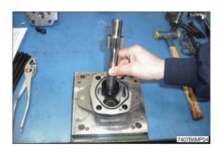
(5) Assemble driven gear. Spread hydraulic fluid around gear set.
