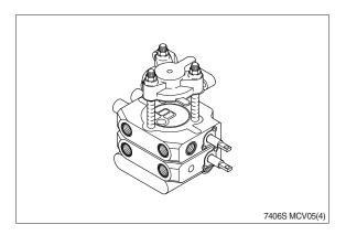
(5) Position valve assembly with the mounting pads of the end sections on a flat surface. To obtain proper alignment of end sections relative to the spool sections apply downward pressure to the end sections; Snug tie rod nuts to about 10 lbf · ft.
