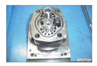
(10) Assemble thrust plate.
