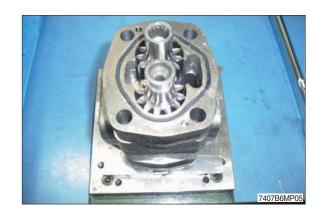
(6) Assemble thrust plate.
