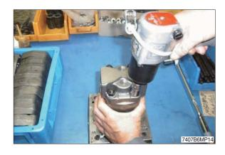
(15) Use torque wrench to assemble.  $\cdot$  Tightening torque : 15 kgf  $\cdot$  m (108 lbf  $\cdot$  ft)
