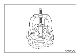
(13) Disassemble the guide of control piston (Mounting position: pilot valve side).
