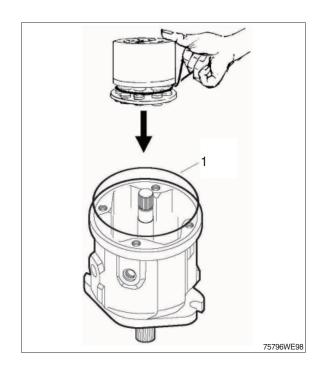
(7) Fit bearing (1) in connection plate.
