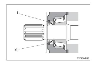
(2) Change the shaft seal and check its sliding surface (drive shaft) and housing, grease the sealing ring.
