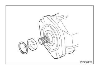
(8) Remove the drive shaft through rear side.
