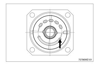
(10) Fit connection plate and control valve.
