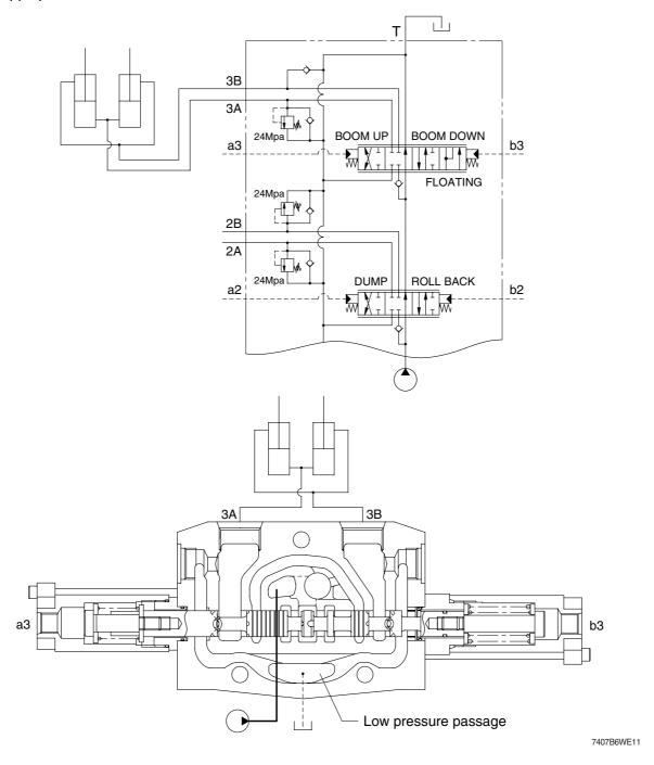
If the remote control valve is not operated, the oil supplied from the pump port passes through the neutral passage to the low pressure passage at the outlet section, and then returns to the tank port.
