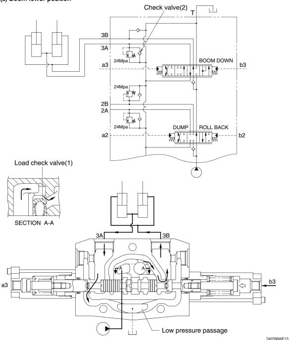
When the pilot pressure from remote control valve is supplied to the pilot port (b3), the spool moves to the left and the neutral passage is closed.
