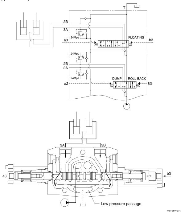
If the remote control lever pushes further more, the pilot pressure from remote control valve rises over 13-15bar and then the boom lowering spool is pushed to the boom floating position, opening up the neutral passage to tank and simultaneously (3A), (3B)  $\rightarrow$  T.
