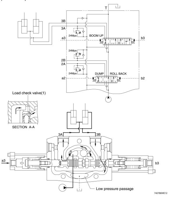
When the pilot pressure from remote control valve is supplied to the pilot port (a3), the spool moves to the right and the neutral passage is closed.
